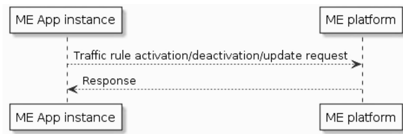
Figure 5.2.7-1: Flow of traffic rule activation/deactivation/update
