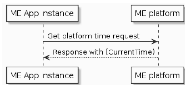
Figure 5.2.10.2-1: Flow of Mobile Edge application requesting platform time
