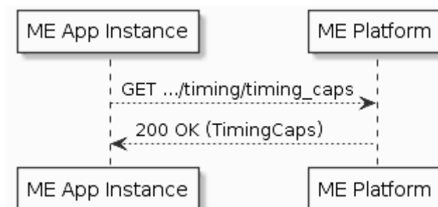
Figure 7.7.3.1-1: GET timing capabilities flow
