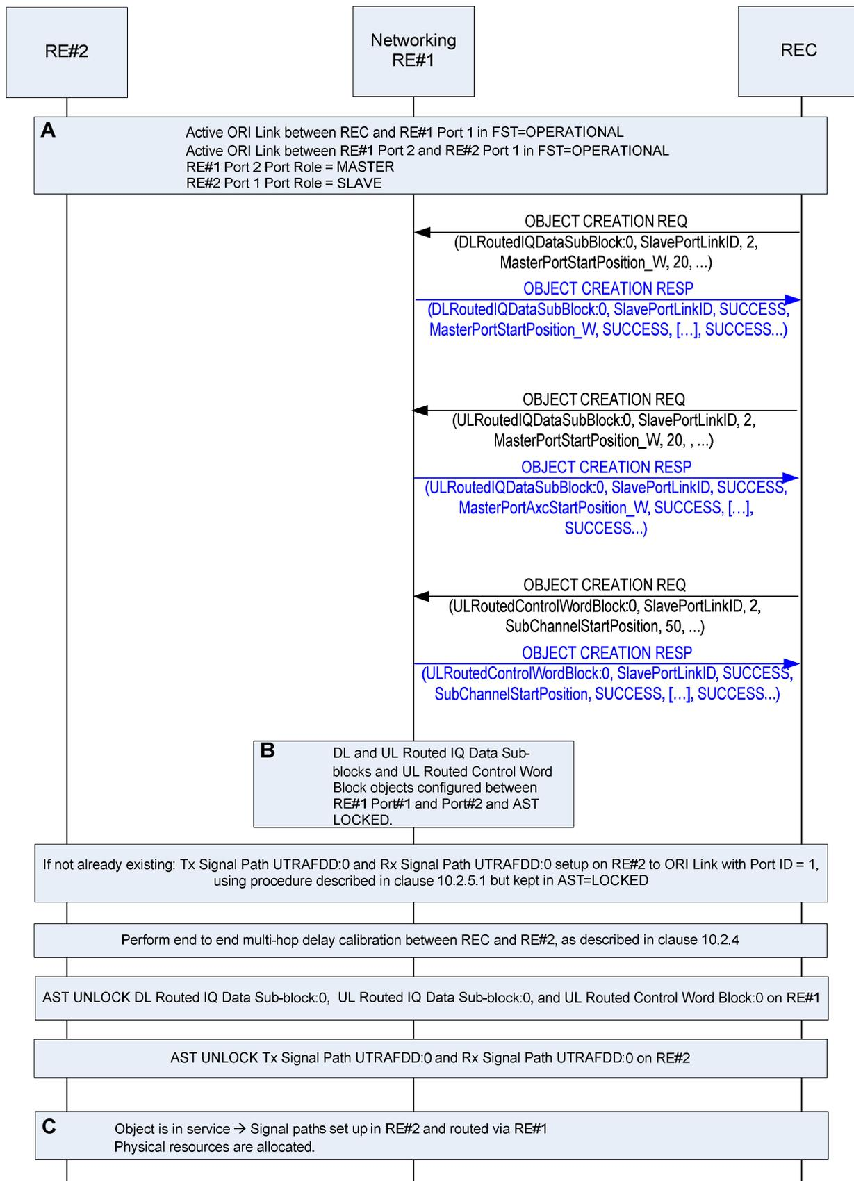
**Figure 10.2.7.3-1: Sequence successful IQ data and control word routing configuration in networking RE in multi-hop configuration**
