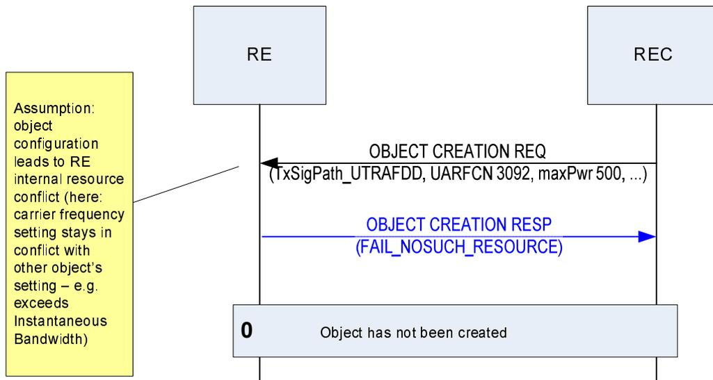
**Figure 10.2.5.1-2: Sequence signal path setup failure**
