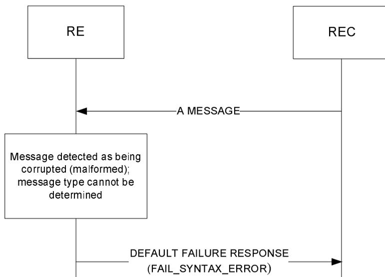
Figure 7.5-1: Default failure response upon malformed message
