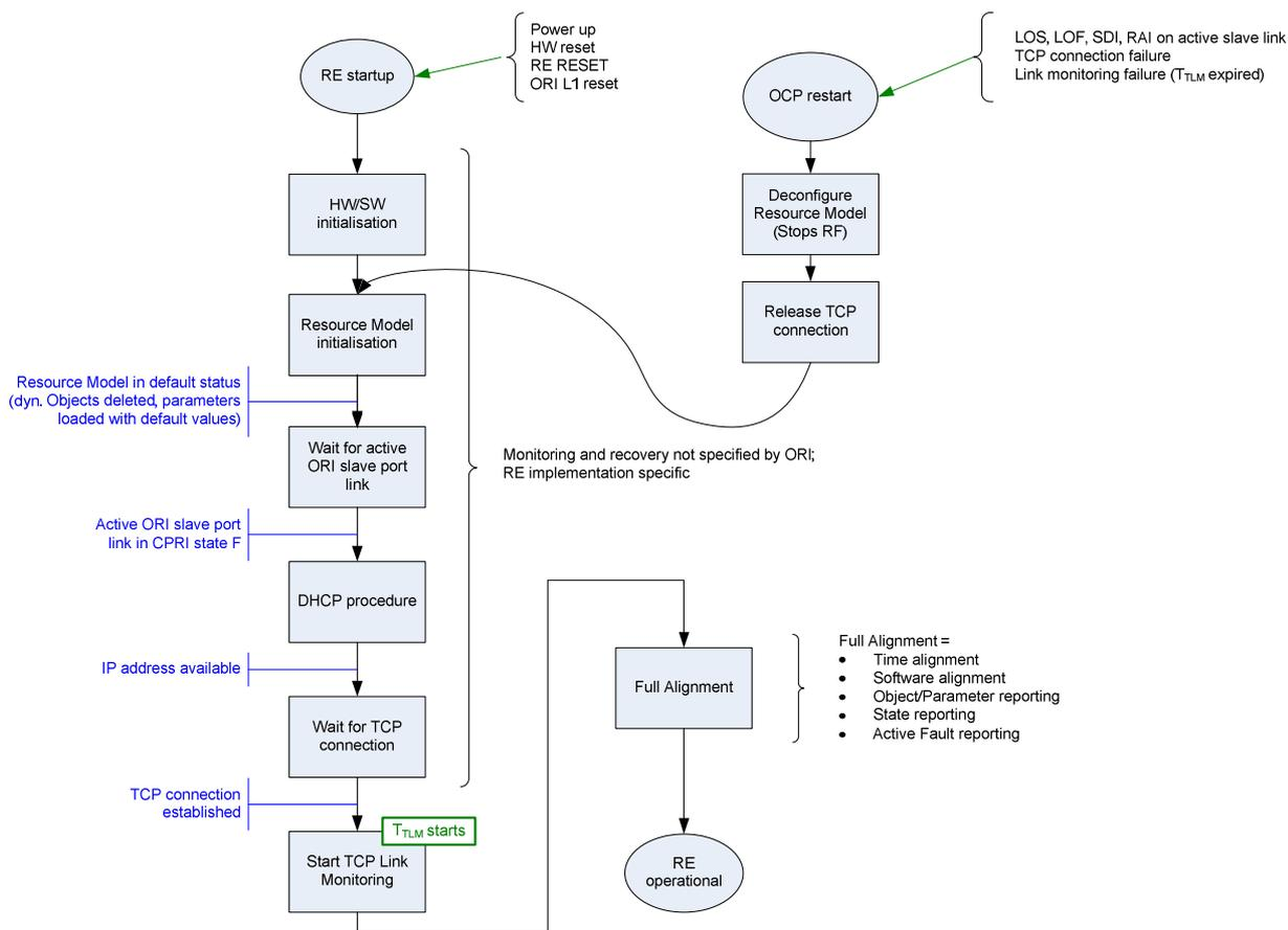
**Figure 10.1.1-1: OCP layer establishment and recovery procedure**
