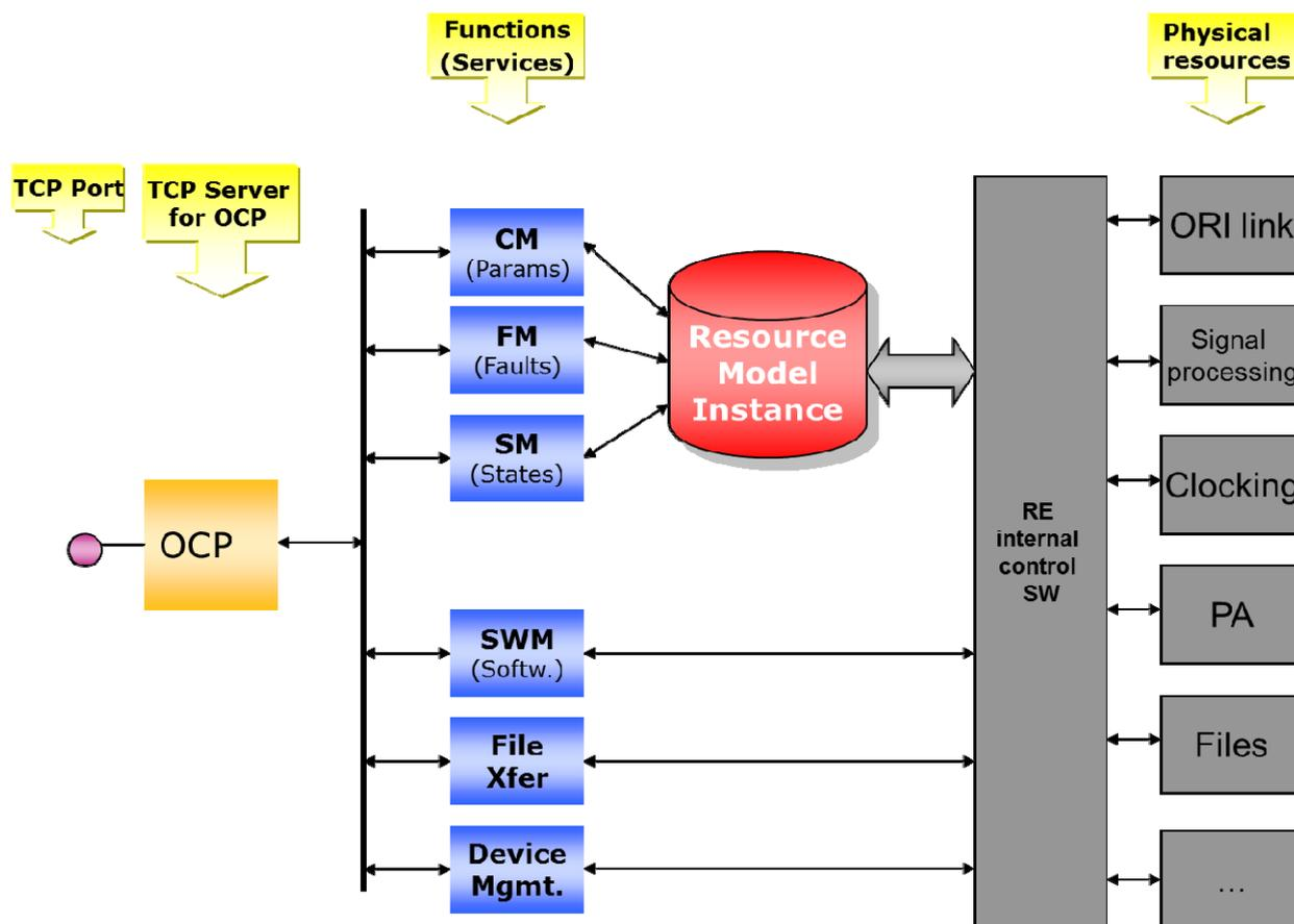
**Figure 6.1-1: System view of the Resource Model**
