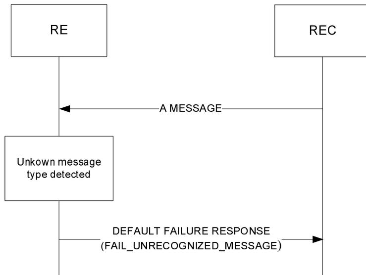
Figure 7.5-2: Default failure response upon unknown message type
