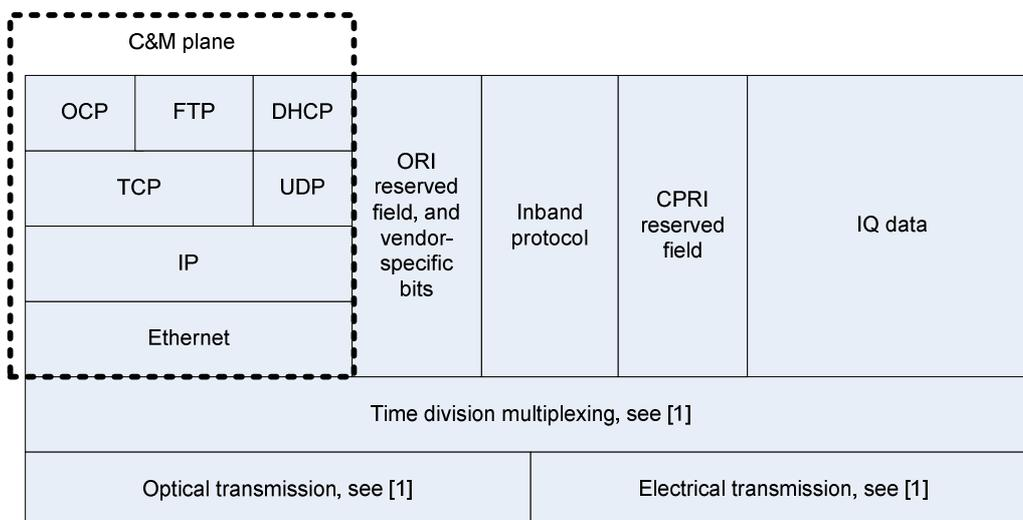
**Figure 5.1-1: ORI protocol stack highlighting C&M plane**
