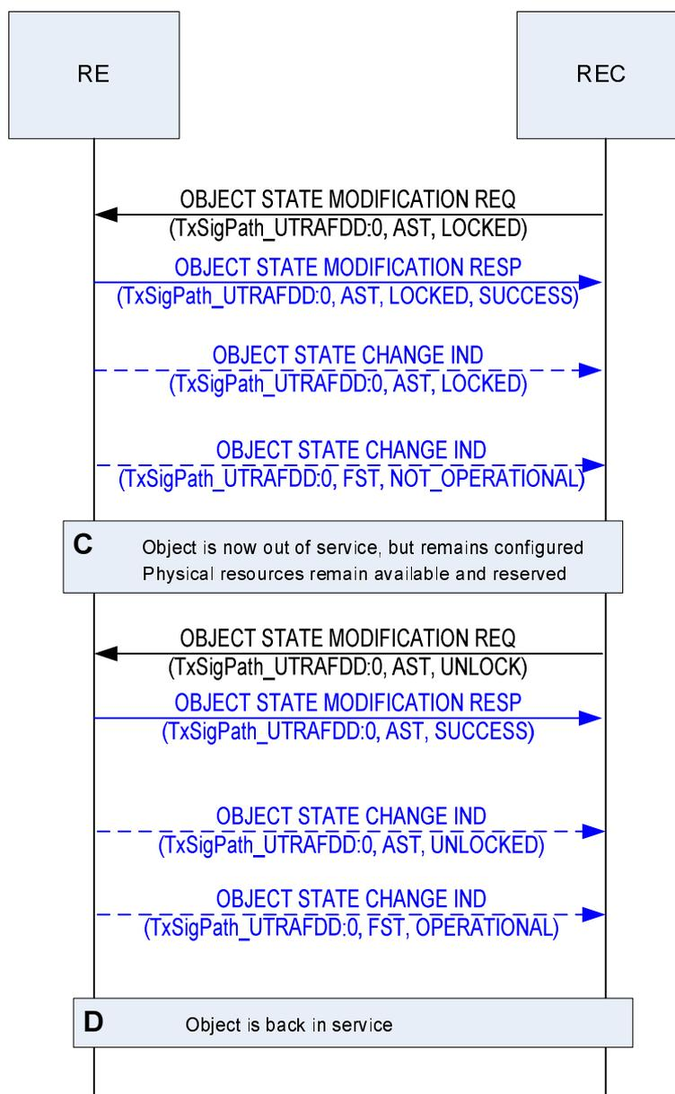
Figure 10.2.5.5-1: Sequence signal path on / off
