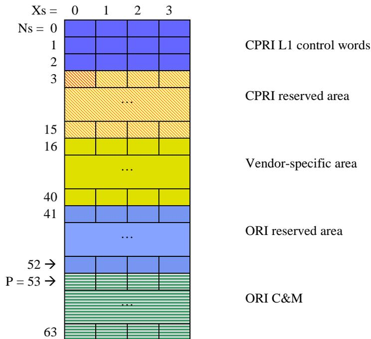
**Figure 6.1.1: Control word mapping to subchannel allocation**
