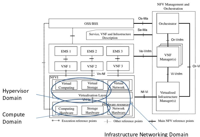
**Figure 1: General Domain Architecture and Associated Interfaces**
