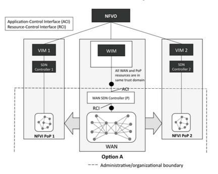
Figure 14: A Single SDN Controller for the WAN Resources (Option A)
