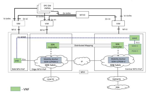
Figure A.14: POC#34 SDN enabled Virtual EPC Gateway
