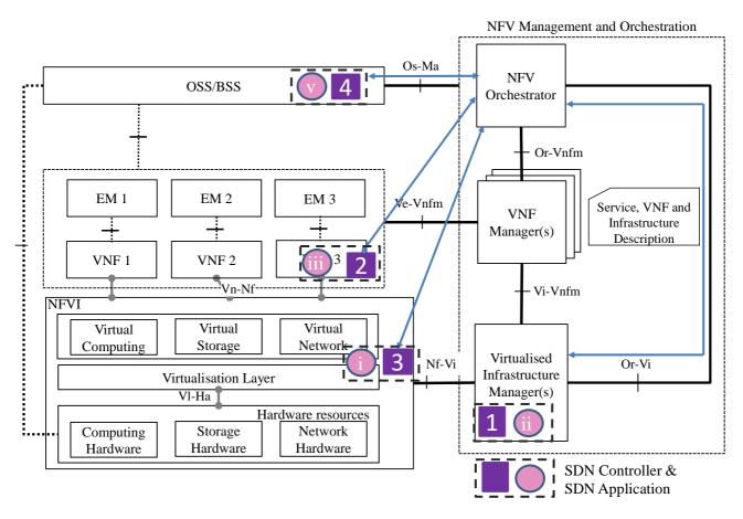
Figure 7: SDN Controller/Application Orchestration Interface Options
