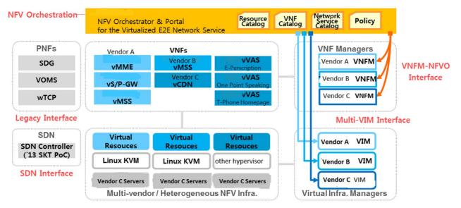
Figure A.10: POC#23 E2E orchestration of Virtualised LTE Core-Network functions
