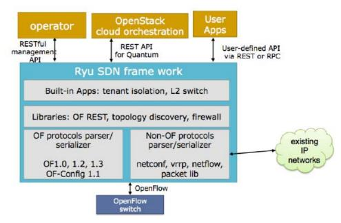
Figure C.5: Ryu SDN Controller architecture overview
