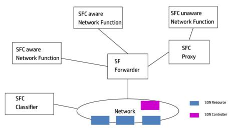
Figure 31: Adding SDN to SFC Underlying Network
