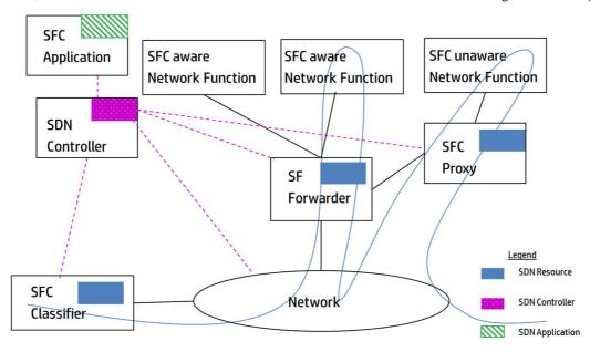
Figure 33: Traffic Flow with SFC and SDN
