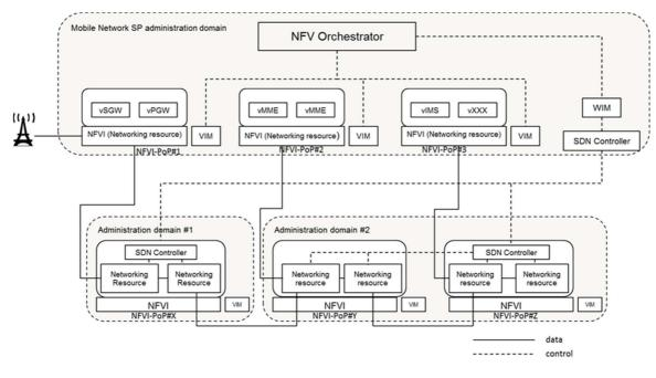
Figure 19: The Mobile Network Scenario for SDN based NaaS Provided by Other Administration Domain
