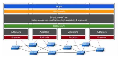
Figure C.8: ONOS SDN Controller architecture overview
