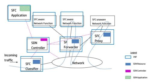
Figure 34: Virtualisation of the SFC Functions with SDN Controller as a VNF
