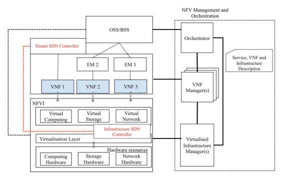
Figure 28: Positioning Infrastructure and Tenant SDN Controllers in the NFV Architecture
