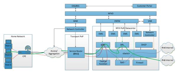
Figure B.6: vCPE Solution architecture - Parental Control use case
