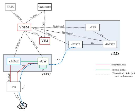
Figure A.12: POC#27 VoLTE Service based on vEPC and vIMS architecture
