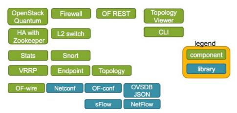
Figure C.6: Ryu SDN controller software components
