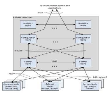
Figure C.4: OpenContrail SDN Controller system implementation
