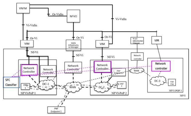
Figure 42: SFC in the NFVI with SDN and NFV in a Multi-Domain, Scalable Environment
