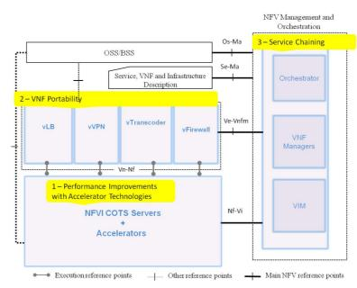
Figure A.9: POC#21 network intensive and compute intensive hardware acceleration
