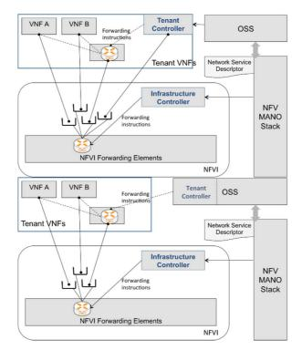
Figure 29: Deployment Options for the Tenant Controller
