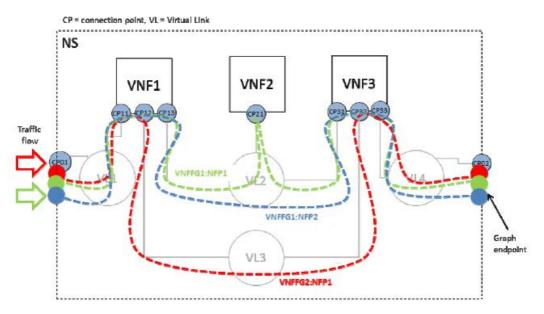
Figure 11: Network Service as defined in figure 6.5 in MANO GS [i.2]
