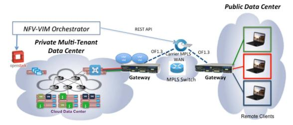
Figure A.7: POC#16 NFVIaaS with Secure SDN-controlled WAN Gateway
