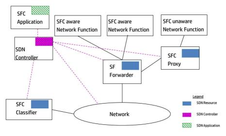
Figure 32: Adding SDN to SFC Components
