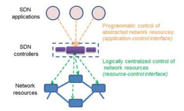
Figure 1: Concept of SDN (from Recommendation ITU-T Y. 3300 [i.8])
