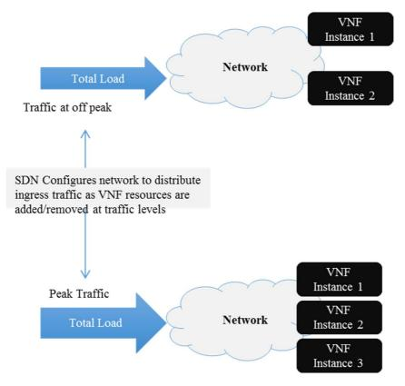
Figure 12: Load Balancing Across VNFs
