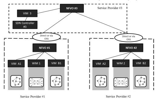
Figure 27: SDN Controller of a Service Provider #3, Across Multiple Service Providers
