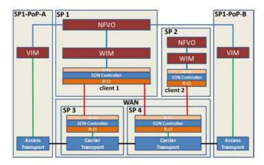
Figure 22: SDN Hierarchy for Different SP
