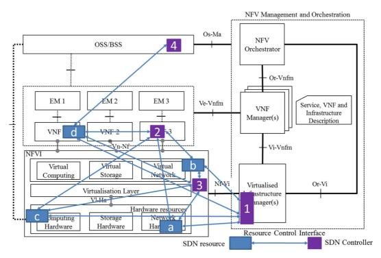
Figure 6: SDN Resource Control Interface Options in NFV
