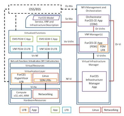
Figure A.5: POC#14 Forces applicability for NFV and integrated SDN
