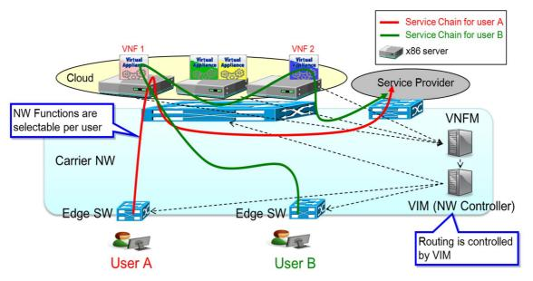
Figure A.2: POC #2 Service Chaining for NW function selection in Carrier Networks
