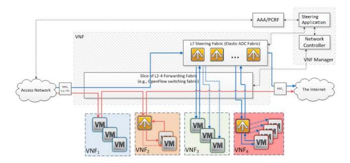
Figure A.4: POC#13 Multi-Layered Traffic Steering for Gi-Lan
