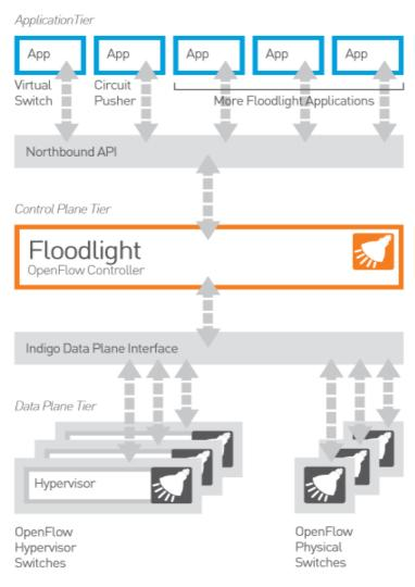
Figure C.1: Floodlight SDN controller architecture overview
