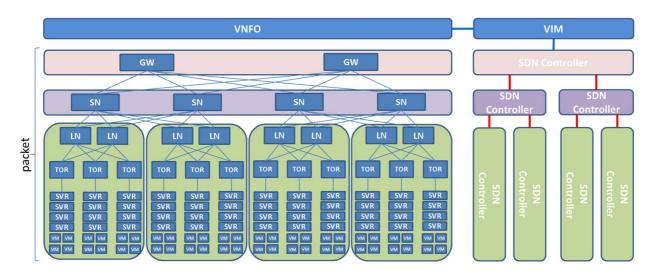
NOTE 1: GW - Gateway, SN - Spine Node, LN - Leaf Node, TOR - Top of the Rack, SVR - Server, VM - Virtual Machine.
