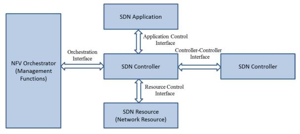
Figure 5: SDN Controller Interfaces
