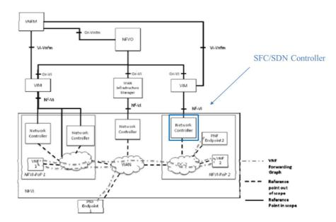
Figure 35: SDN Controller in NFVI (based on MANO [i.2] figure 5.2)
