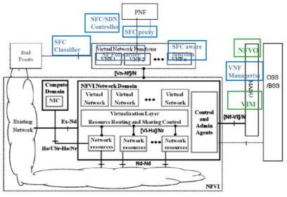
Execution reference points \_\_\_\_\_ Other reference points \_\_\_\_\_ Main NFV reference points
