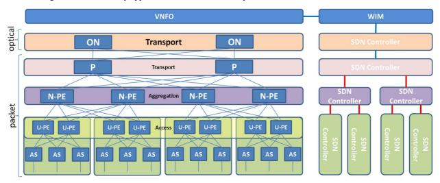
NOTE 1: ON-Optical Node, P - Provider, PE-Provide Edge, N-PE - Network Provide Edge, U-PE - User Provider Edge, AS - Access Switch.
