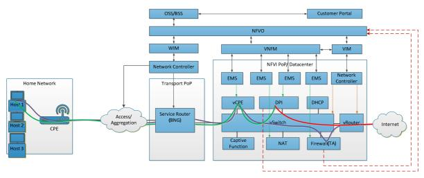
Figure B.7: vCPE Solution architecture - DoS/DdoS protection use case
