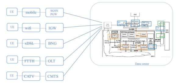
Figure 41: End to End Carrier Network with SFC, SDN, NFV in the Data Center
