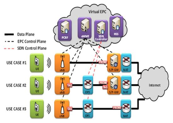
Figure A.11: POC#26 Virtual EPC with SDN functions in Mobile Backhaul Networks
