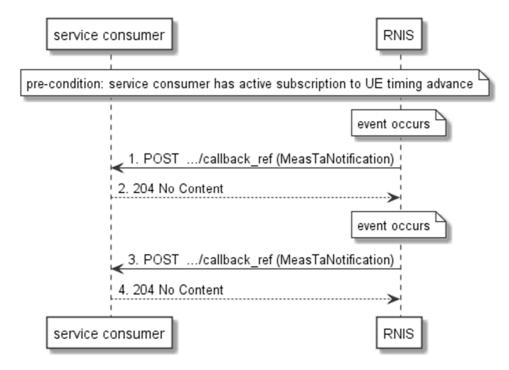
Figure 5.2.11-1: Flow of receiving RNI event notifications on UE timing advance
