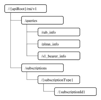
Figure 7.2-1: Resource URI structure of the RNI API
