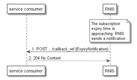
Figure 5.2.5.2-1: Flow of RNIS sending a notification on expiry of the subscription
