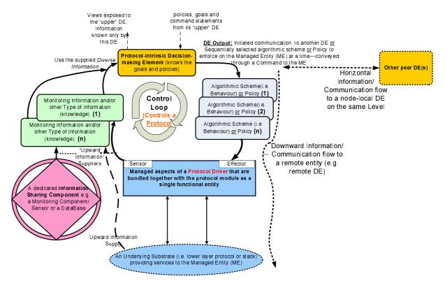
Figure 8: A protocol-intrinsic control-loop
