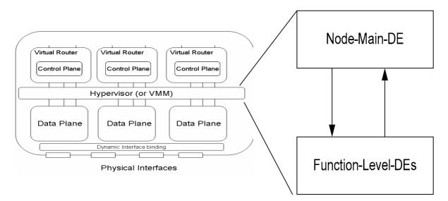
Figure 43: Example of Virtualised Router
