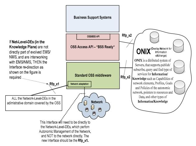
Figure 67: How to integrate an OSS and GANA Network-Level-DEs and the ONIX
