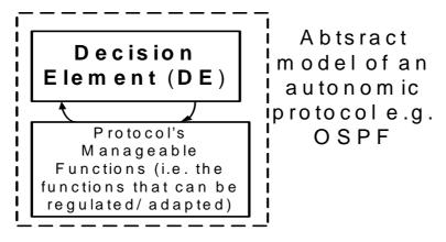
Figure 15: A protocol-intrinsic Control-Loop
