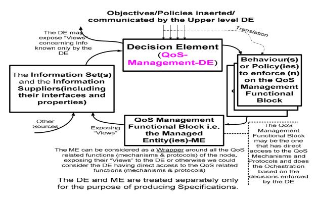
Figure 16: A Control-Loop specific to an abstracted "Networking Function" -QoS Management, and some of the key items that call for "Design Specifications"
