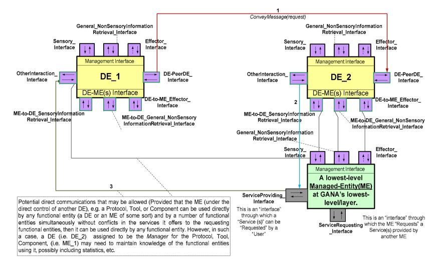
Figure 28: A case in which the DE may need to communicate with an ME that is not its own, via the DE of the ME
