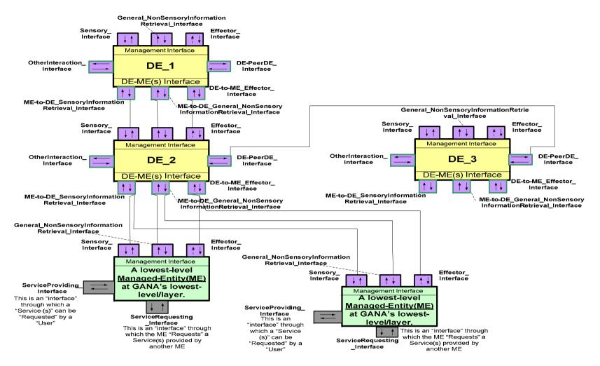
Figure 26: A DE with multiple MEs and interfacing with an Upper and a PeerDE (which could be a sibling DE since a Sibling relation is a special-type of a Peer Relation)
