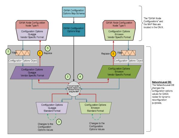
Figure 56: Dynamic reconfiguration of a node by the network-level DEs using vendor specific configuration options and "GANA Configuration options Map"
