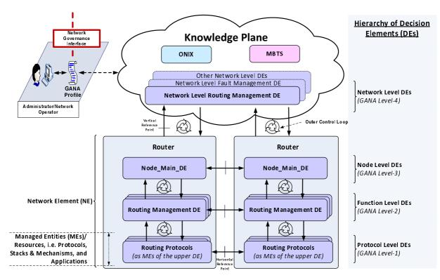
Figure 3: GANA Instantiation within a Router, w.r.t Autonomic Routing Functionality
