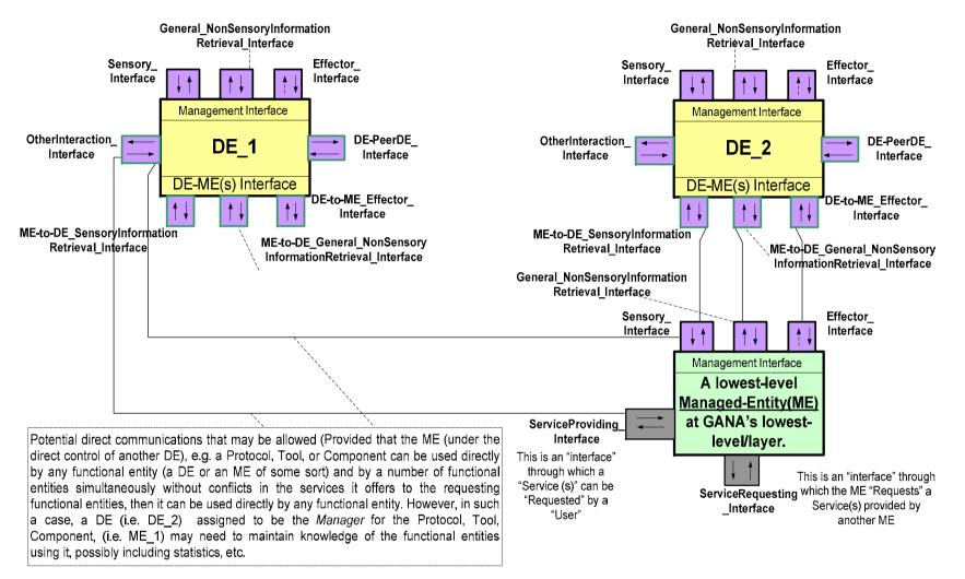
Figure 27: A situation under which a DE is allowed to interact directly with an ME that is not its own
