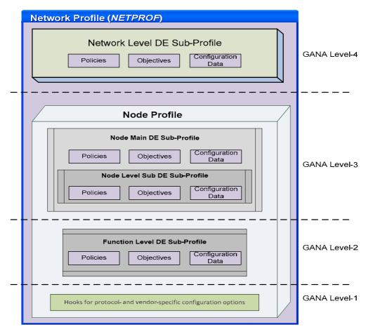
Figure 51: Vertical decomposition of the Network Profile
