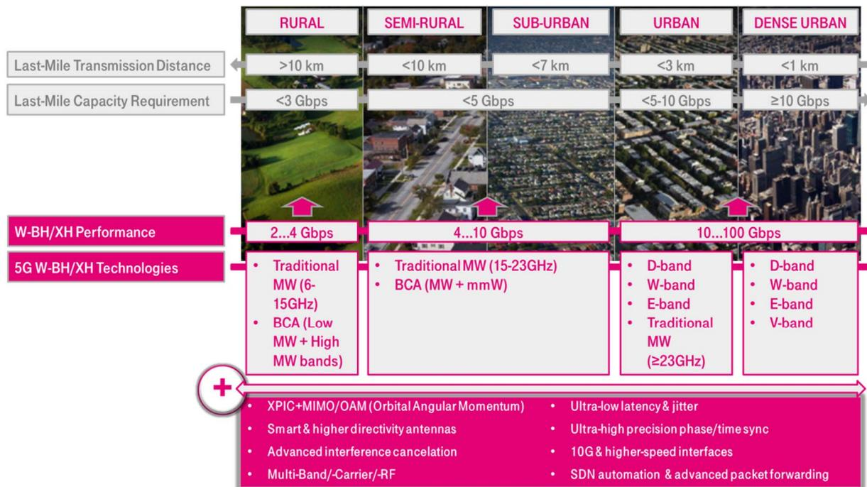
**Figure 11: Wireless Backhaul/X-Haul Technologies Fit 5G**
