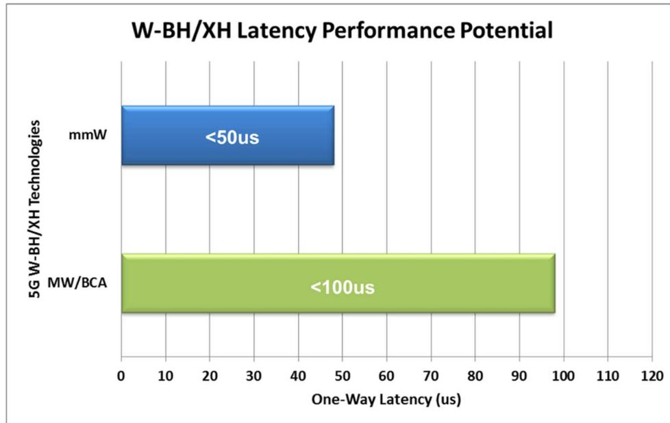
Figure 10: MW Backhaul/X-Haul Technologies Future Latency Performance
