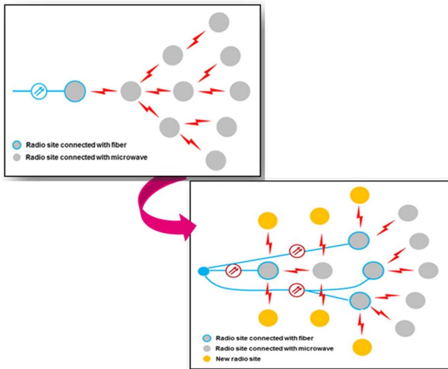
**Figure 6: Macro-Cell Backhaul Network Topologies Shift**
