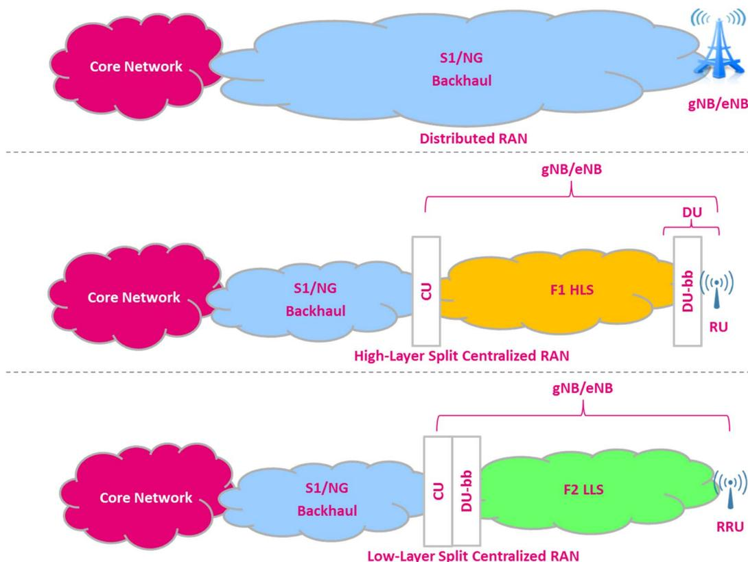
**Figure 5: Distributed and Centralized RAN Architectures**
