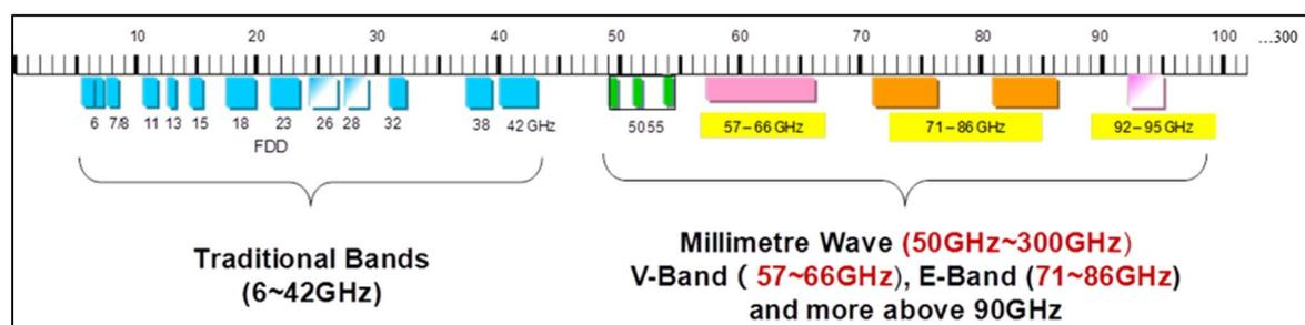
Figure 8: Microwave and Millimetre Wave Spectrum
