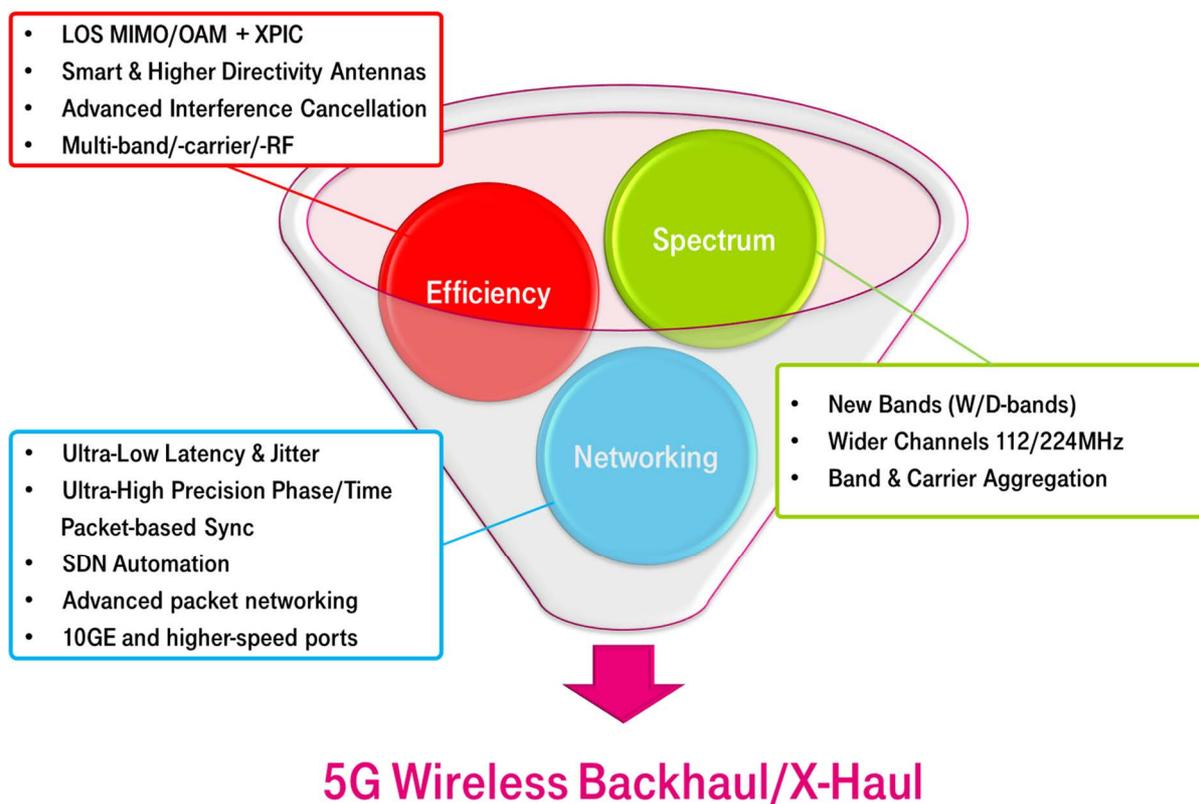
Figure 9: Pillars of 5G Wireless Backhaul/X-Haul Evolution & Innovation
