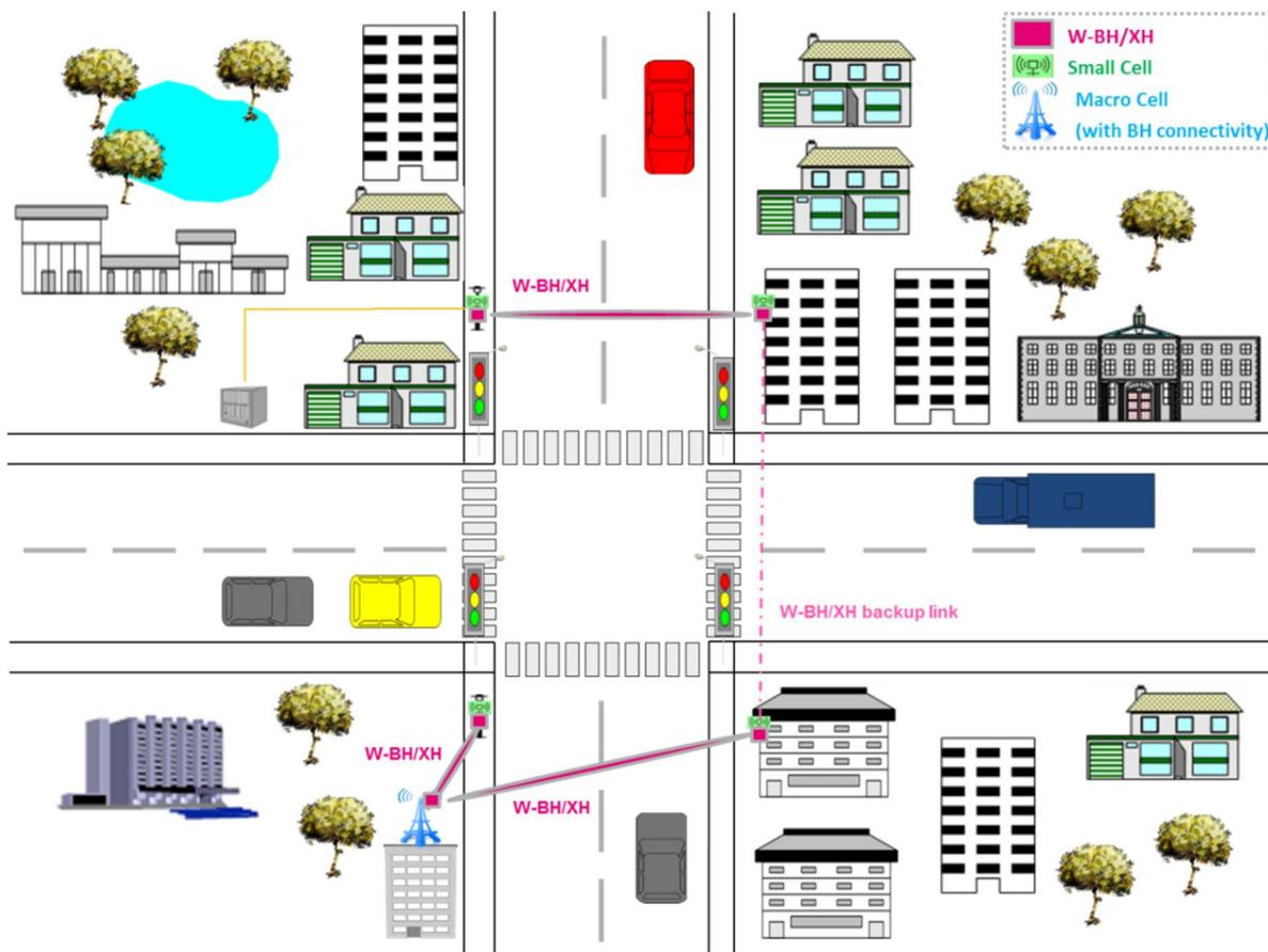
Figure 7: Small-Cell Backhaul/X-Haul Network Topologies
