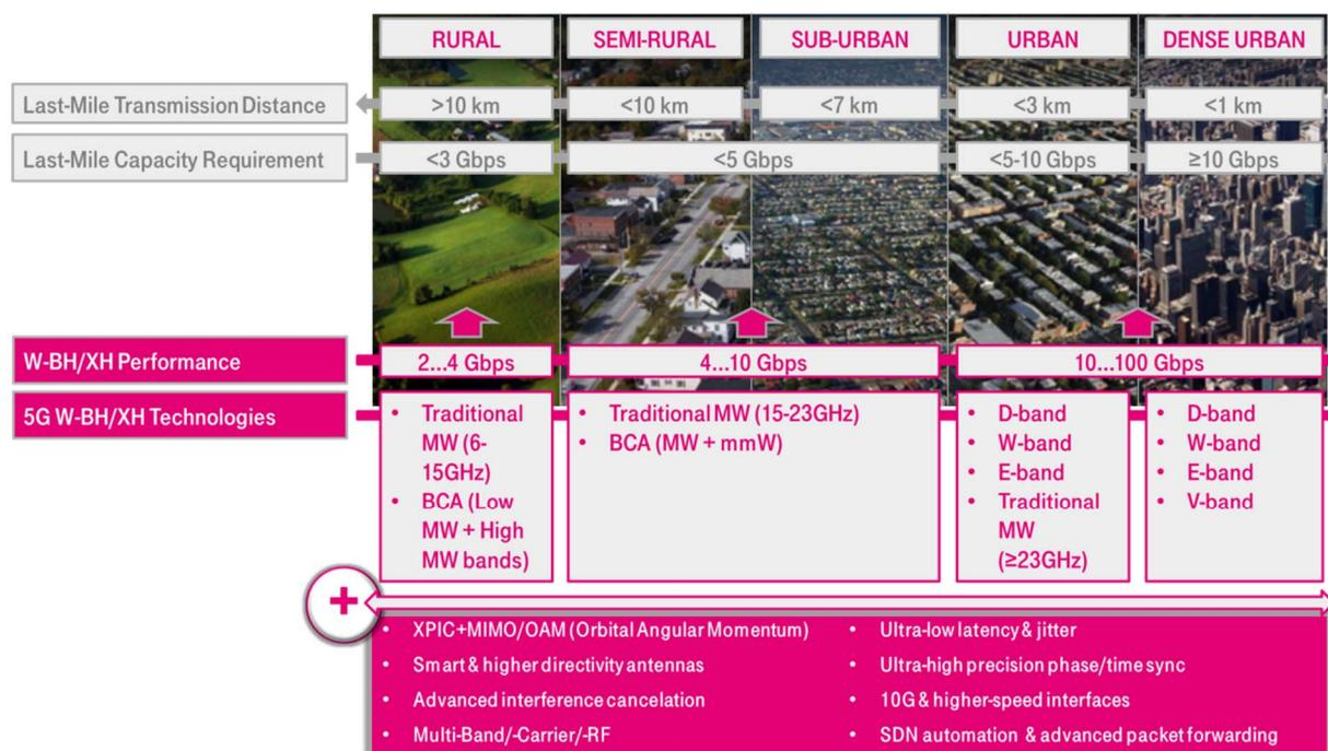
**Figure 11: Wireless Backhaul/X-Haul Technologies Fit 5G**
