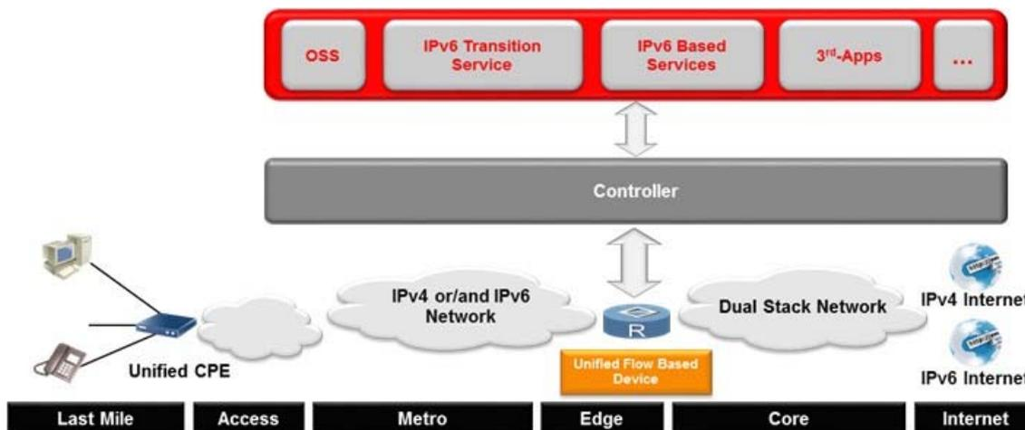
**Figure 1: Overall Architecture of IPv6-based SDN solution**
