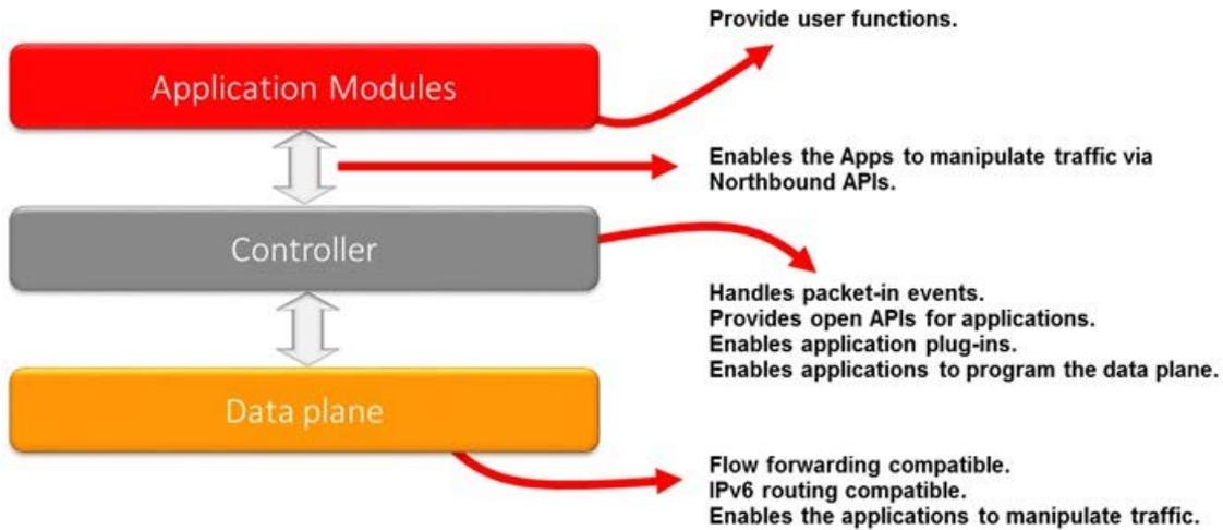
**Figure 2: Layered Architecture of IPv6-based SDN solution**
