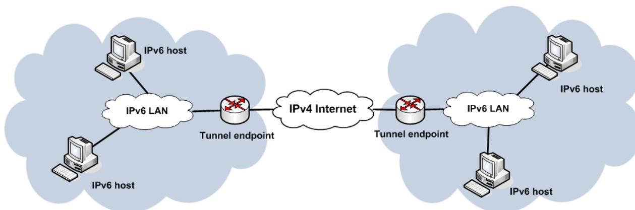
Figure 2: Typical 6in4 tunnel scenario
