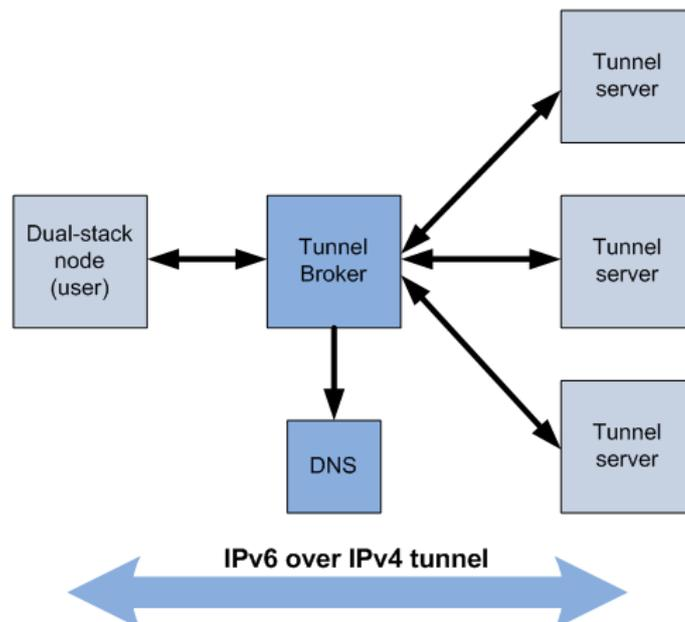
Figure 7: Architecture of a possible Tunnel Broker deployment
