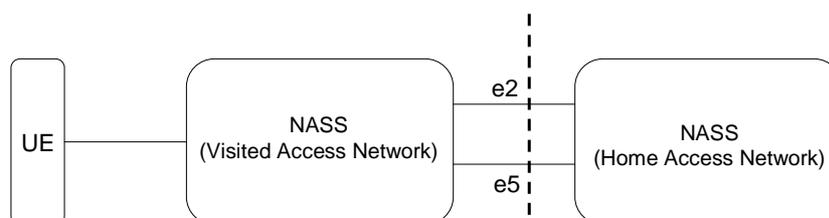
**Figure 6: Network interconnection at the NASS level**
