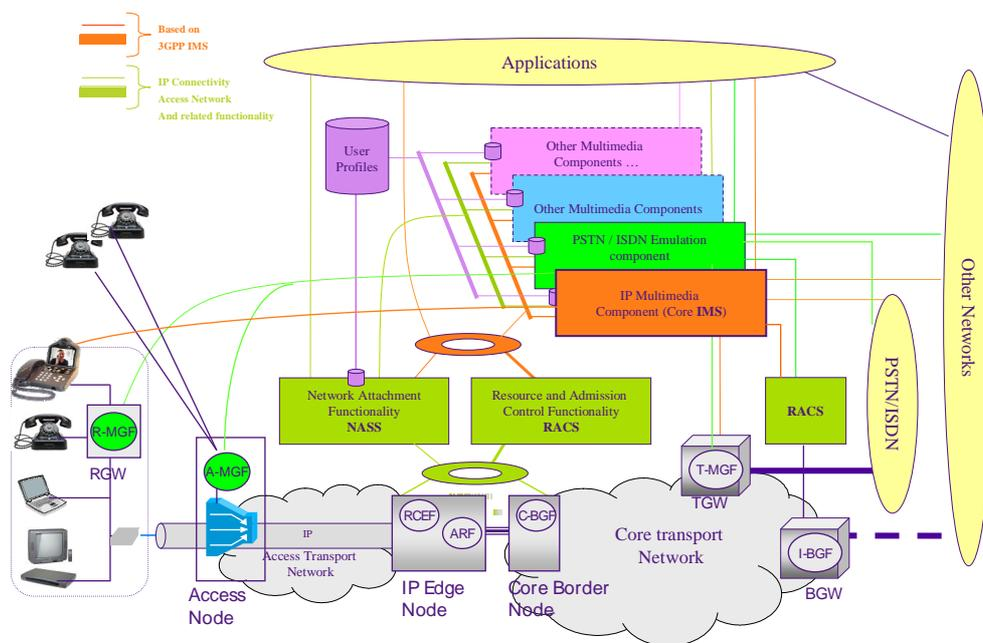
**Figure A.1: Example architecture with xDSL access**
