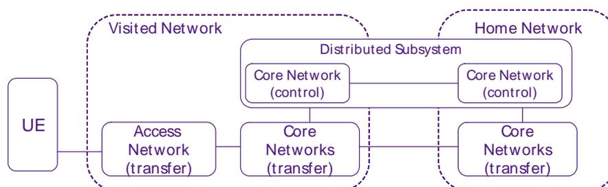
**Figure 2: Distributed subsystems**
