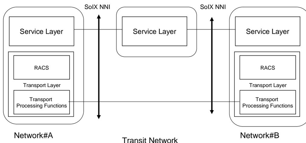
**Figure 7i: Indirect Interconnection with service layer intermediary**
