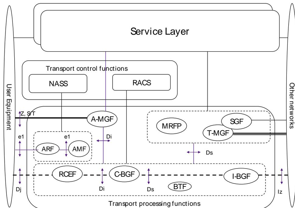
**Figure 3: Transport processing functions overview**
