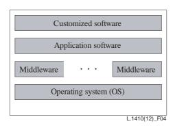
Figure 6: Software structure of an ICT system (example)
