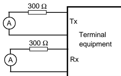
**Figure A.11: Power feeding test for 4 wire TE****Interface state:**
