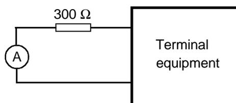
**Figure A.10: Power feeding test for 2 wire TE**
