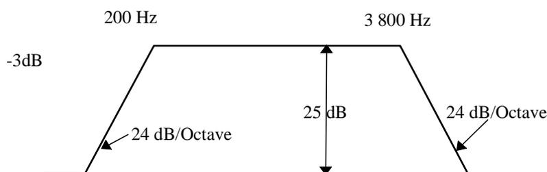
Figure A.1: Response for the band-limiting filter
