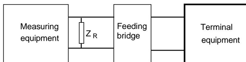
**Figure A.5: Mean sending level configuration**
