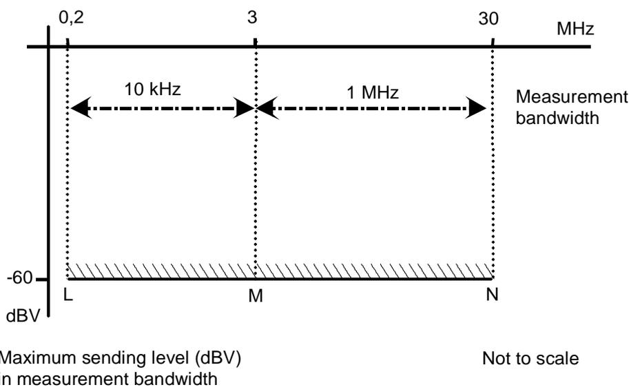
Figure 5: Maximum sending between 200 kHz and 30 MHz
