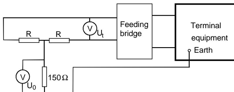
**Figure A.4: Output Signal Balance certification****DC feeding arrangement:**
