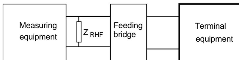
**Figure A.9: Sending level between 200 kHz and 30 MHz configuration****DC feeding arrangement:**
