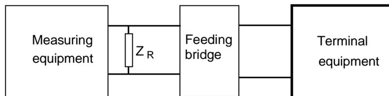
**Figure A.8: Sending level between 4,3 kHz and 200 kHz configuration****DC feeding arrangement:**
