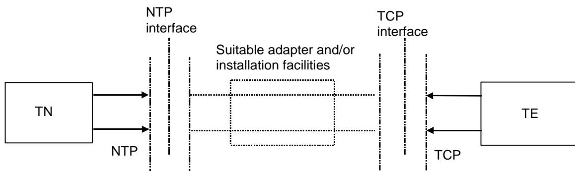
**Figure 1: Terminal connection point and network termination point**
