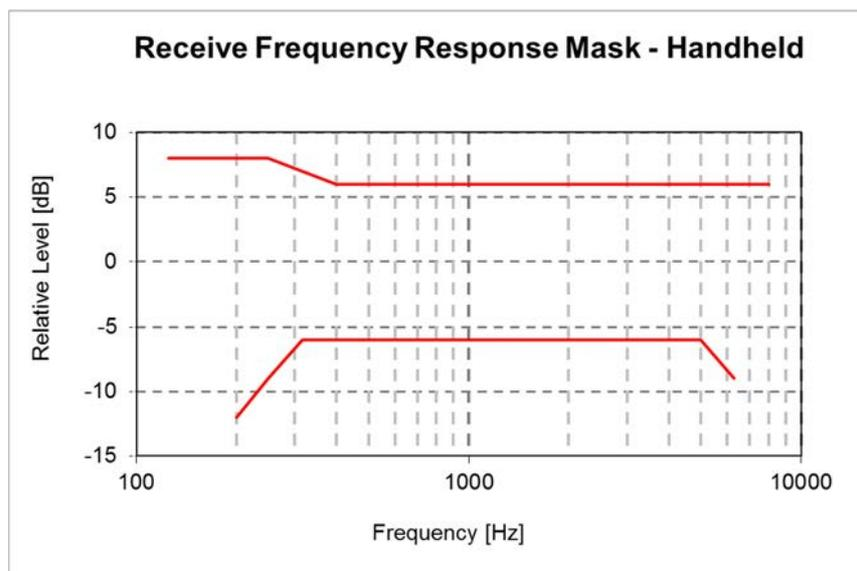
Figure 15: Receive frequency response mask for Hand-held HFT
