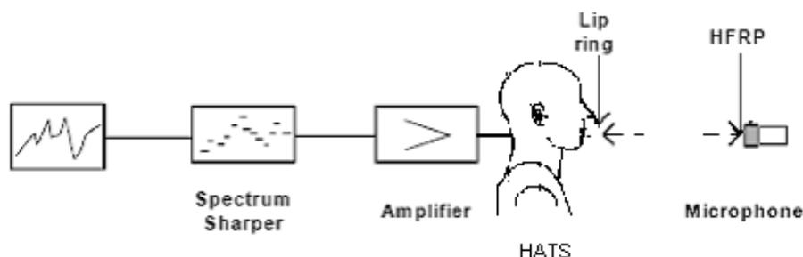
Figure 11: Calibration at HFRP (with  $d_{HFS} = 50$  cm)
