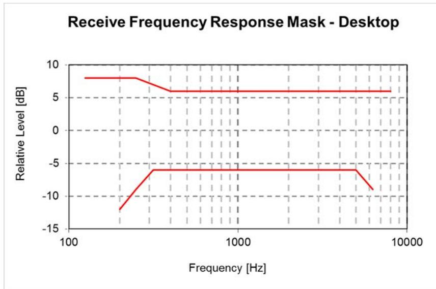
Figure 14: Receive frequency mask for Desktop HFT
