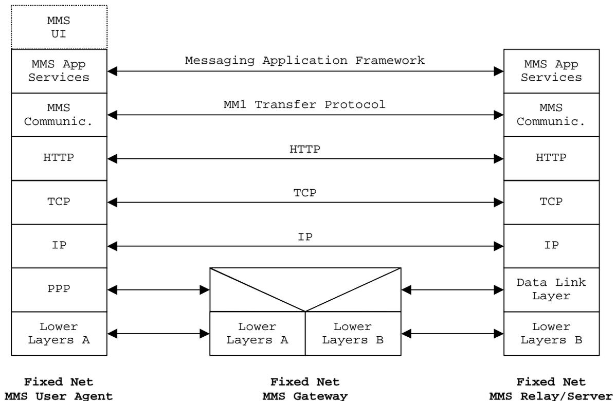
**Figure 11: MM1 protocol layers in fixed networks for MM submission, MM retrieval, MM read report (recipient side) and MM forwarding**
