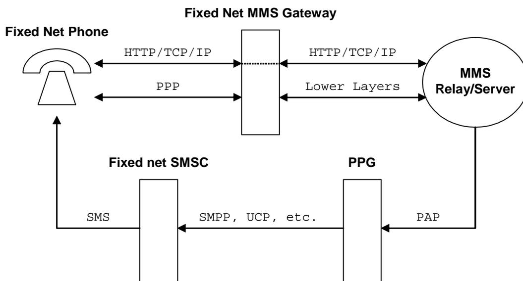
Figure 3: General MM1 gateway structure for fixed networks
