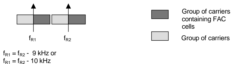
Figure K.6: Example of base/enhancement DRM signals
