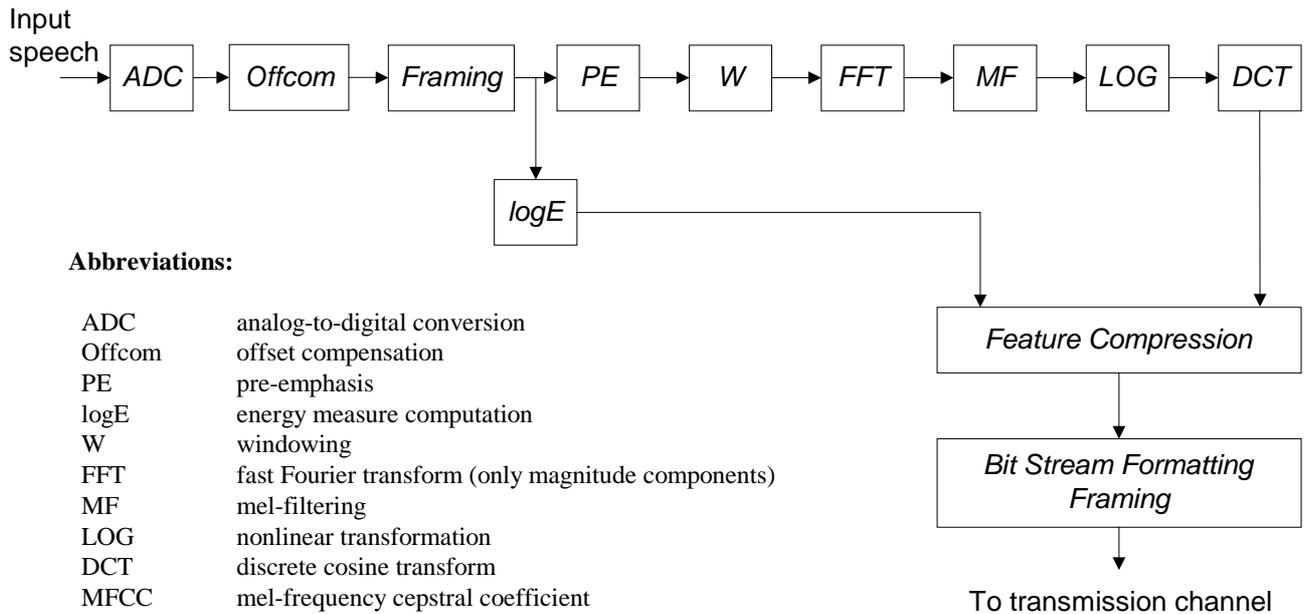
**Figure 4.1: Block diagram of the front-end algorithm**
