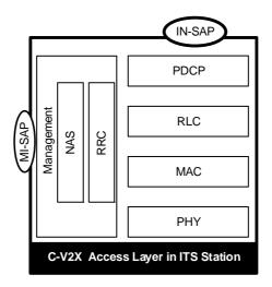
Figure 4.1-2: LTE-V2X Access Layer protocol stack
