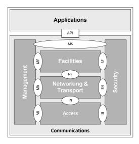
Figure 4.1-1: ITS station architecture
