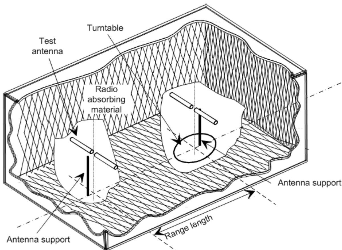
**Figure A.1: A typical anechoic chamber**
