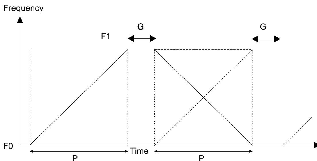
Figure E.2: Typical FMCW modulation scheme
