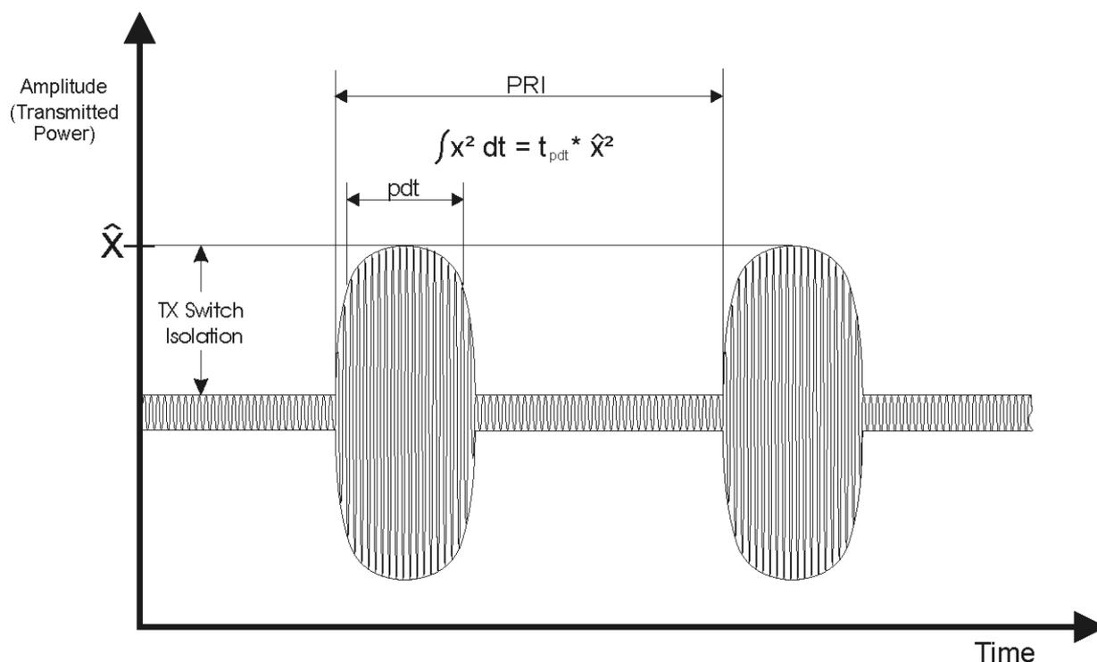
Figure E.6: Typical pulse modulation scheme
