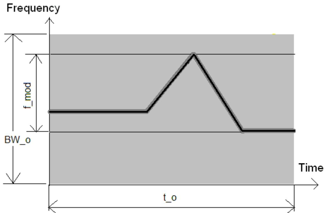
NOTE: Colour denotes signal power, reading modulation frequency range.
