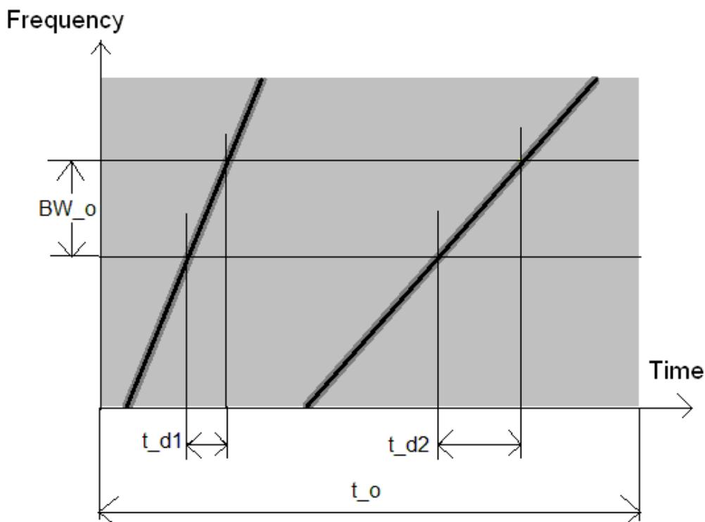
NOTE: Grey-scale denotes signal power, two individual dwell time contributions for accumulation over a given observation bandwidth  $BW_o$  and of a given observation time  $t_o$ .
