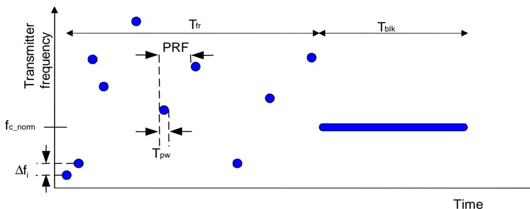
Figure E.7: Typical Pulsed FH Modulation
