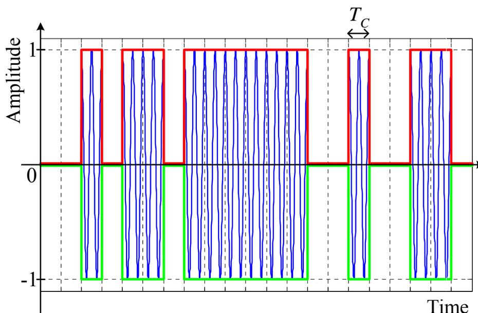
Figure E.5: Typical PN-ASK modulation scheme
