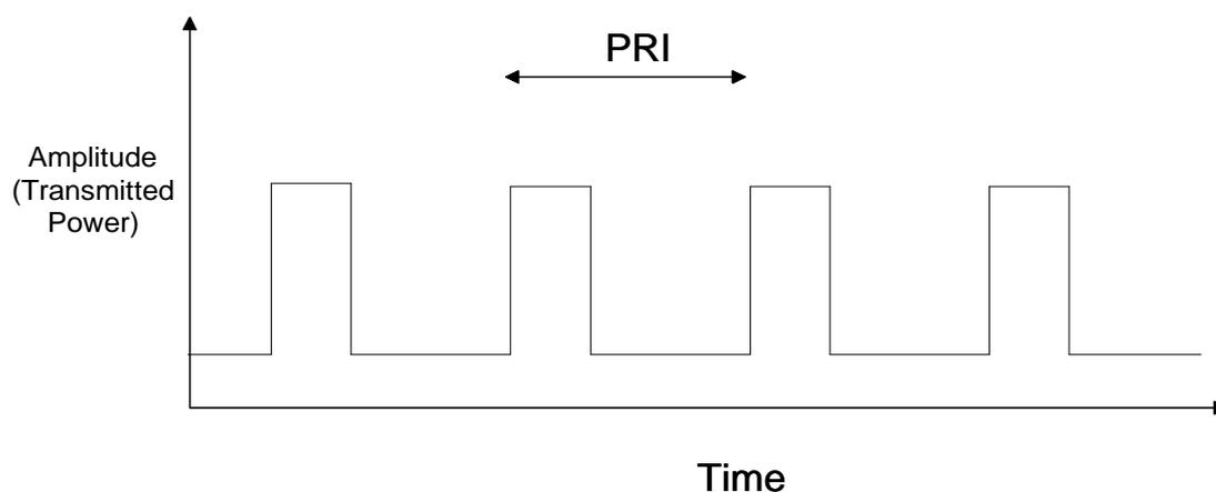
Figure E.1: Typical pulse modulation scheme
