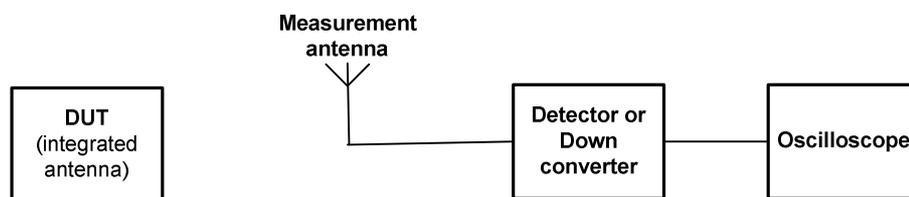
**Figure 3: General test setup to execute the time domain procedure for DC measurement in the case of radiated emission**
