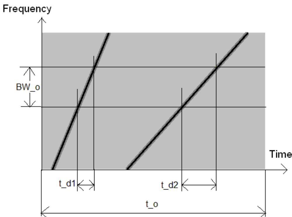
NOTE: Grey scale denotes signal power, two individual time contributions occur for a given observation bandwidth  $BW_o$  and over a given observation time interval  $t_o$ .
