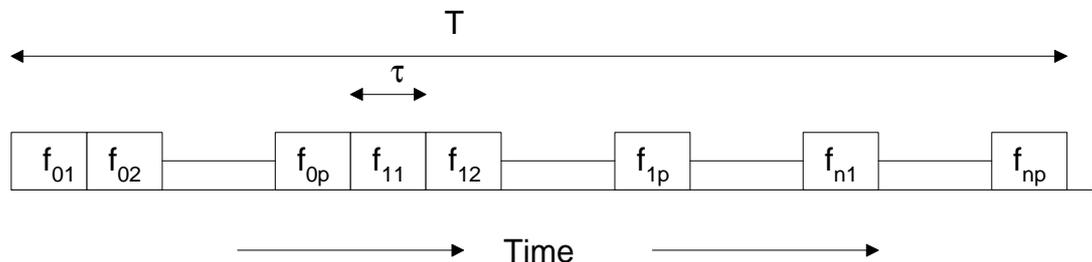
Figure E.3: Typical FSK modulation scheme
