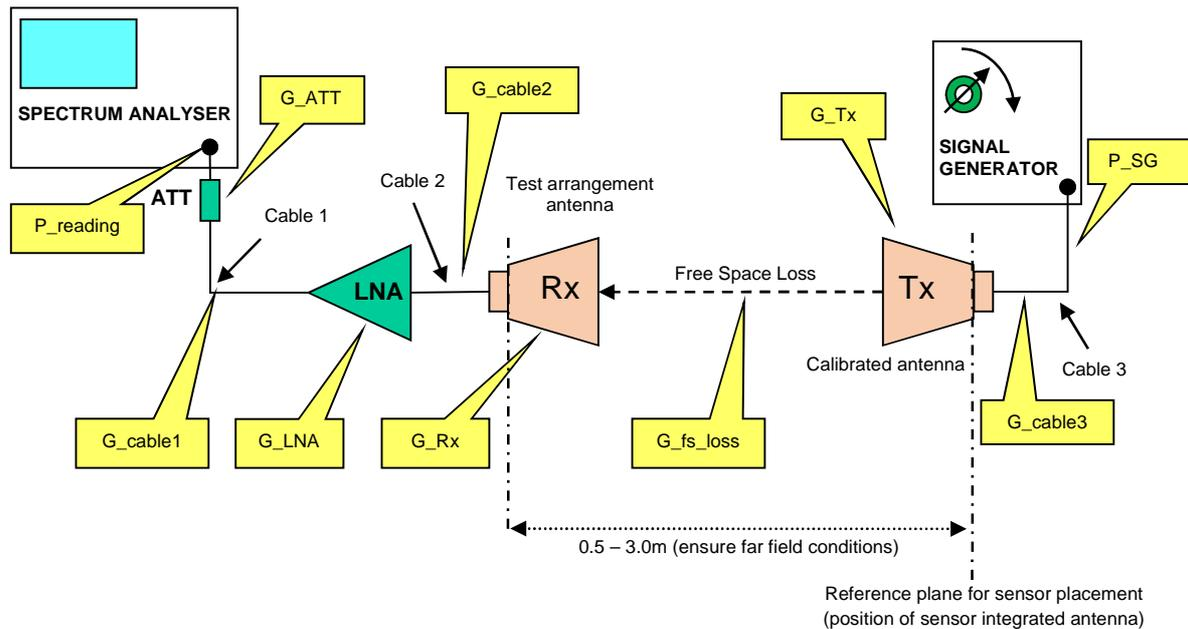
**Figure C.1: Calibration set-up configuration**
