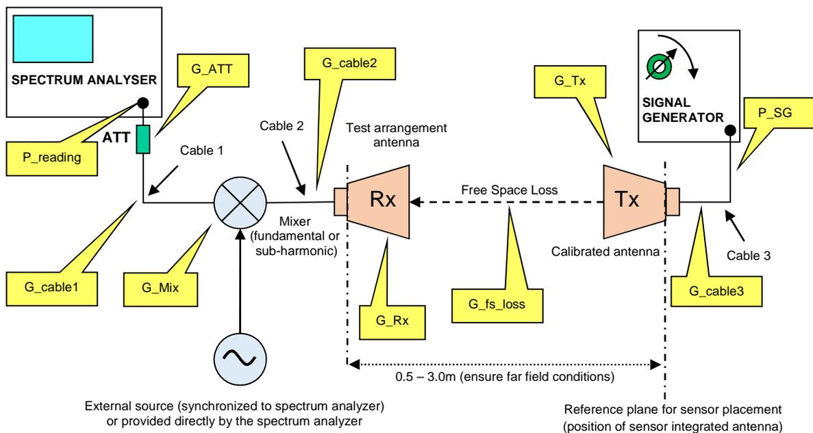
**Figure C.2: Calibration set-up configuration including a mixer**
