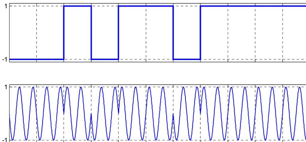
**Figure E.8: Typical binary direct sequence impulse  $c(t)$  and the transmitted PN-2-PSK signal  $s(t)$**
