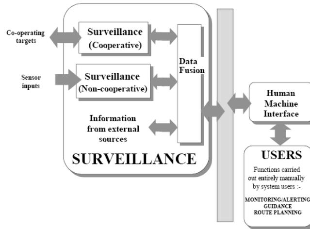
**Figure 1: A-SMGCS Level 1 Functional Configuration**
