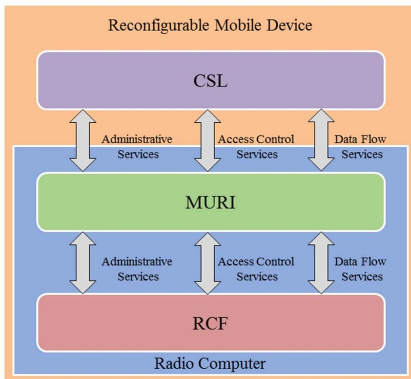
**Figure 5.1: Interconnection between CSL and RCF using MURI for Reconfigurable MD**
