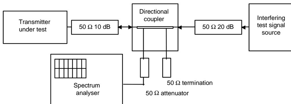
**Figure 5: Measurement arrangement**
