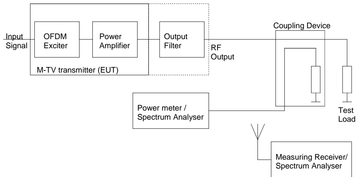
NOTE: If the transmitter does not include any output filter, an external filter shall be added after the transmitter for the testing arrangement. This filter shall be representative of the multiplexer or filter existing in operational conditions and viewed by the transmitted output when installed.
