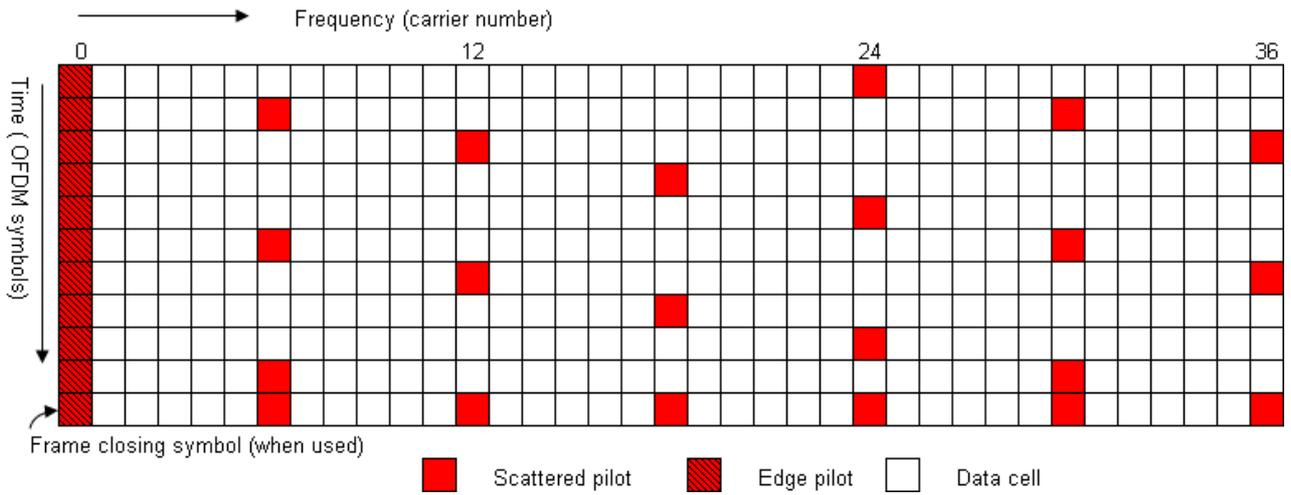
**Figure K.3: Scattered pilot pattern PP3 (SISO)**
