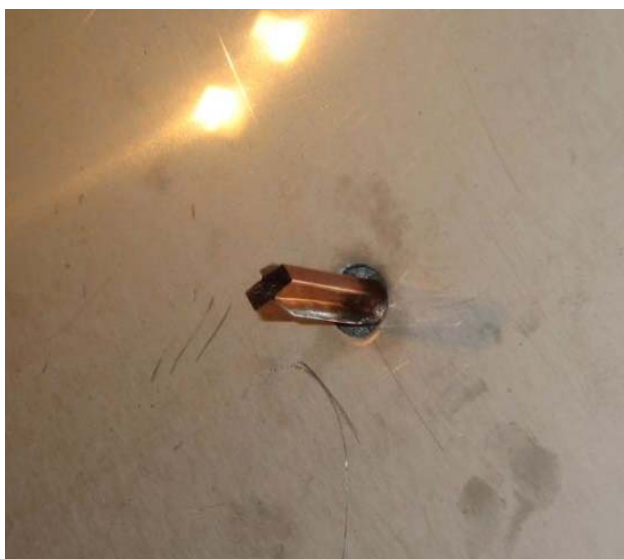
Figure 11: APC measurement setup - Details of open ended waveguide through the metal
