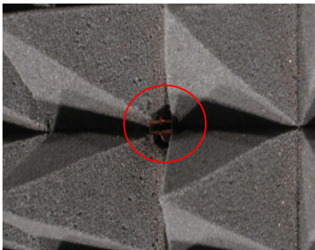
Figure 10: APC measurement setup - open ended waveguide fitted in absorbing foam
