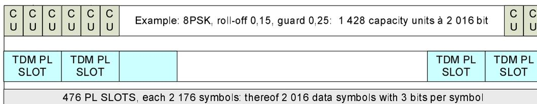
Figure 5.21: Example of TDM frame for 8PSK
