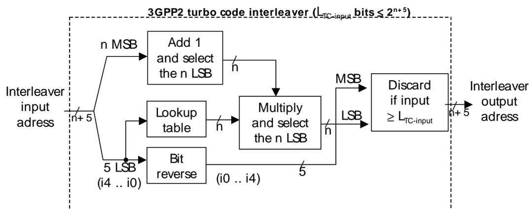
Figure 5.8: Turbo interleaver output address calculation procedure
