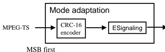
**Figure 5.1: Functional block diagram of the mode adaptation**
