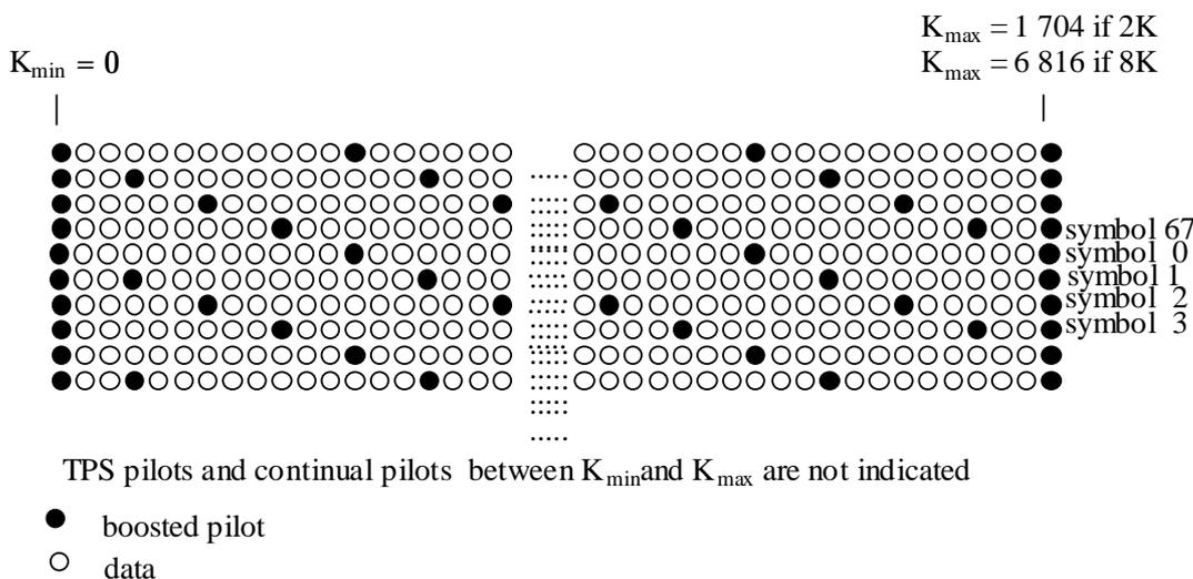
Figure 5.35: Frame structure
