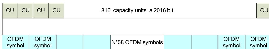
Figure 5.26: Mapping of the SH frame on OFDM
