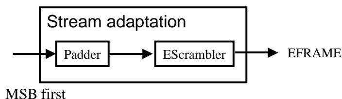
Figure 5.4: Functional block diagram of the stream adaptation
