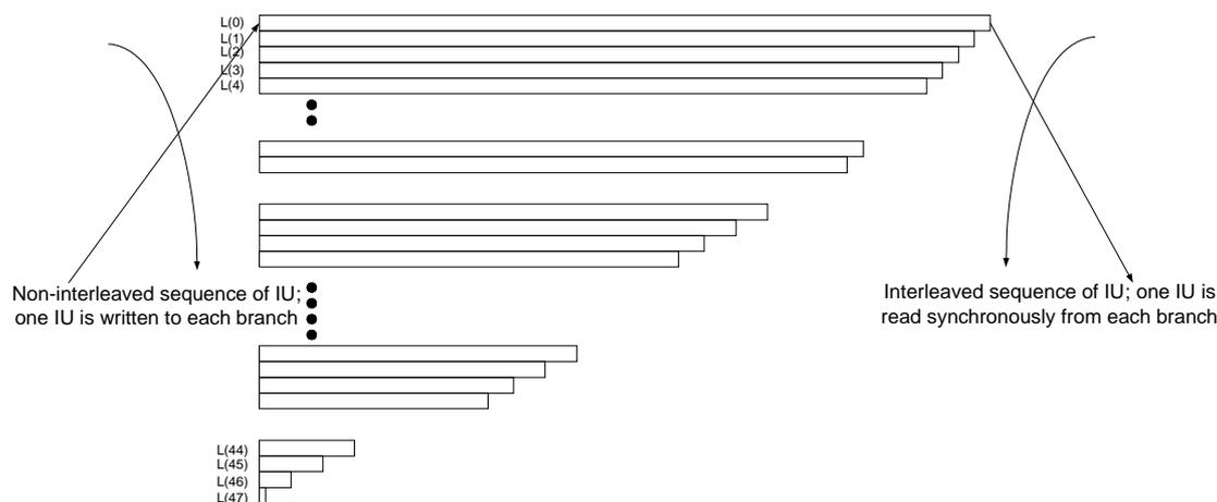
**Figure 5.9: Conceptual diagram of the time interleaver**
