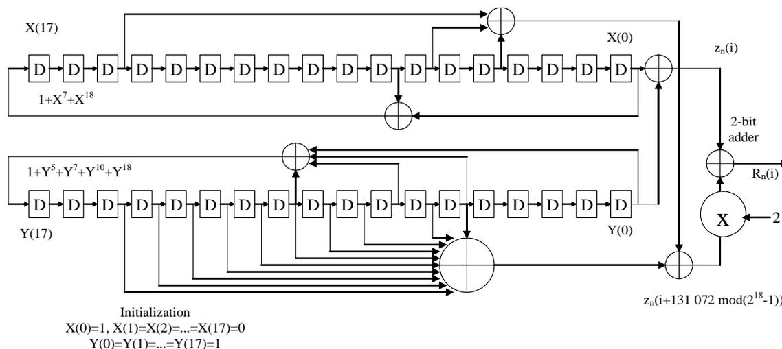
**Figure 5.25: Configuration of PL scrambling code generator**
