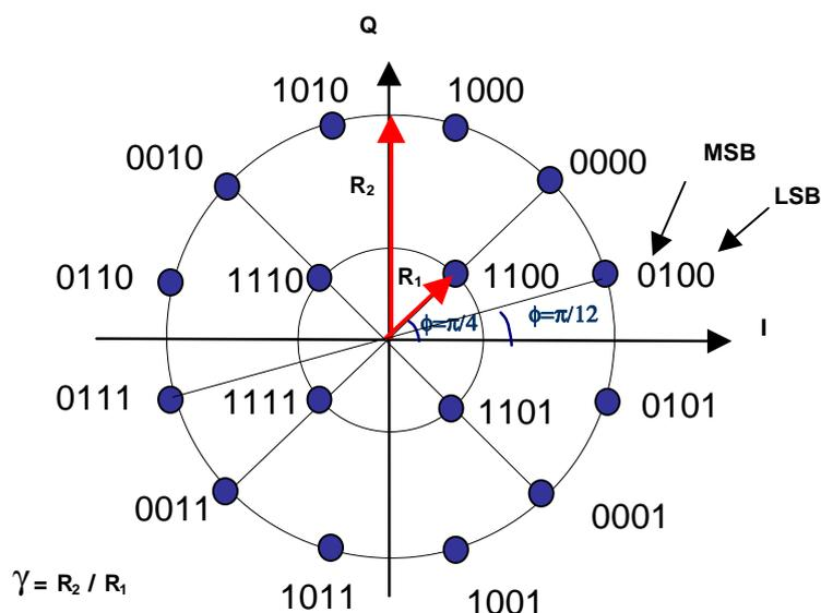
Figure 5.19: Bit mapping into 16APSK signal constellation
