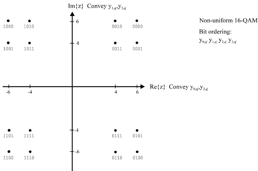
**Figure 5.33: Non-uniform 16-QAM mappings with  $\alpha = 4$**
