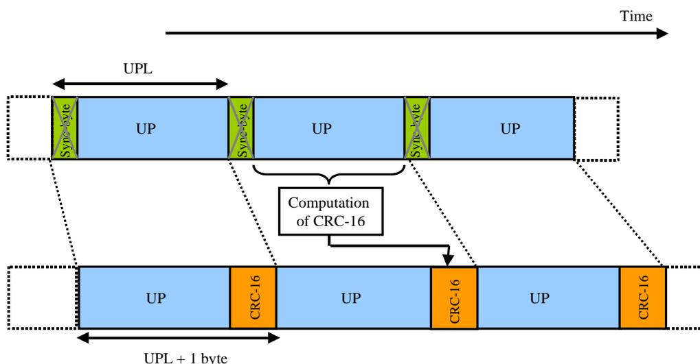
**Figure 5.2: Illustration of the CRC-16 encoding process**
