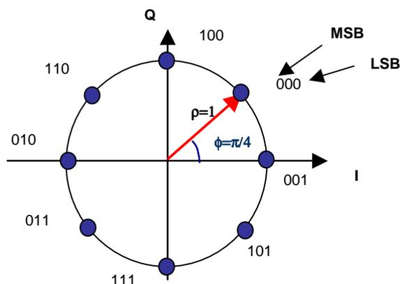
Figure 5.18: Bit mapping into 8PSK constellation
