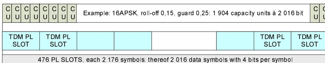
Figure 5.22: Example of TDM frame for 16APSK
