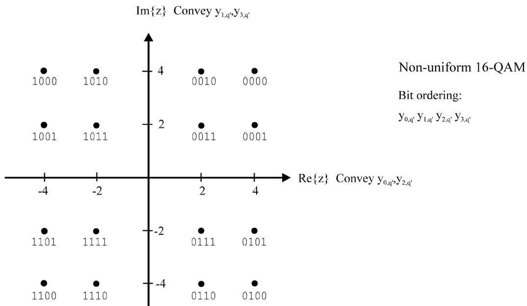
**Figure 5.32: Non-uniform 16-QAM mappings with  $\alpha = 2$**
