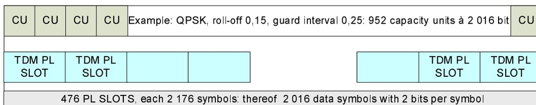
Figure 5.20: Example of TDM frame for QPSK
