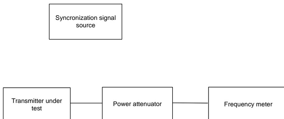
Figure 4: Measurement arrangement
