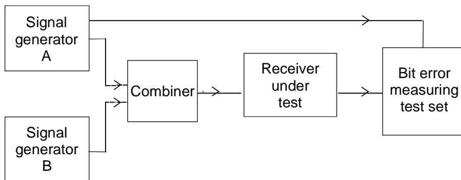
**Figure 9: Measurement arrangement**
