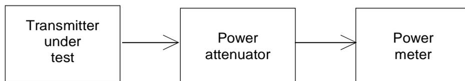
**Figure 1: Measurement arrangement**
