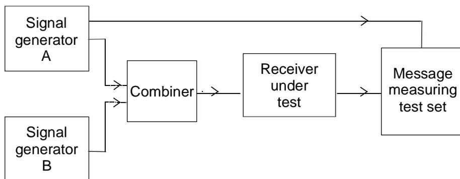
**Figure 8: Measurement arrangement**
