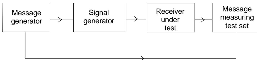
**Figure 6: Measurement arrangement**
