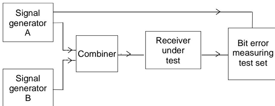
**Figure 7: Measurement arrangement**
