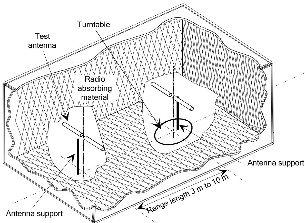
**Figure B.1: A typical anechoic chamber**
