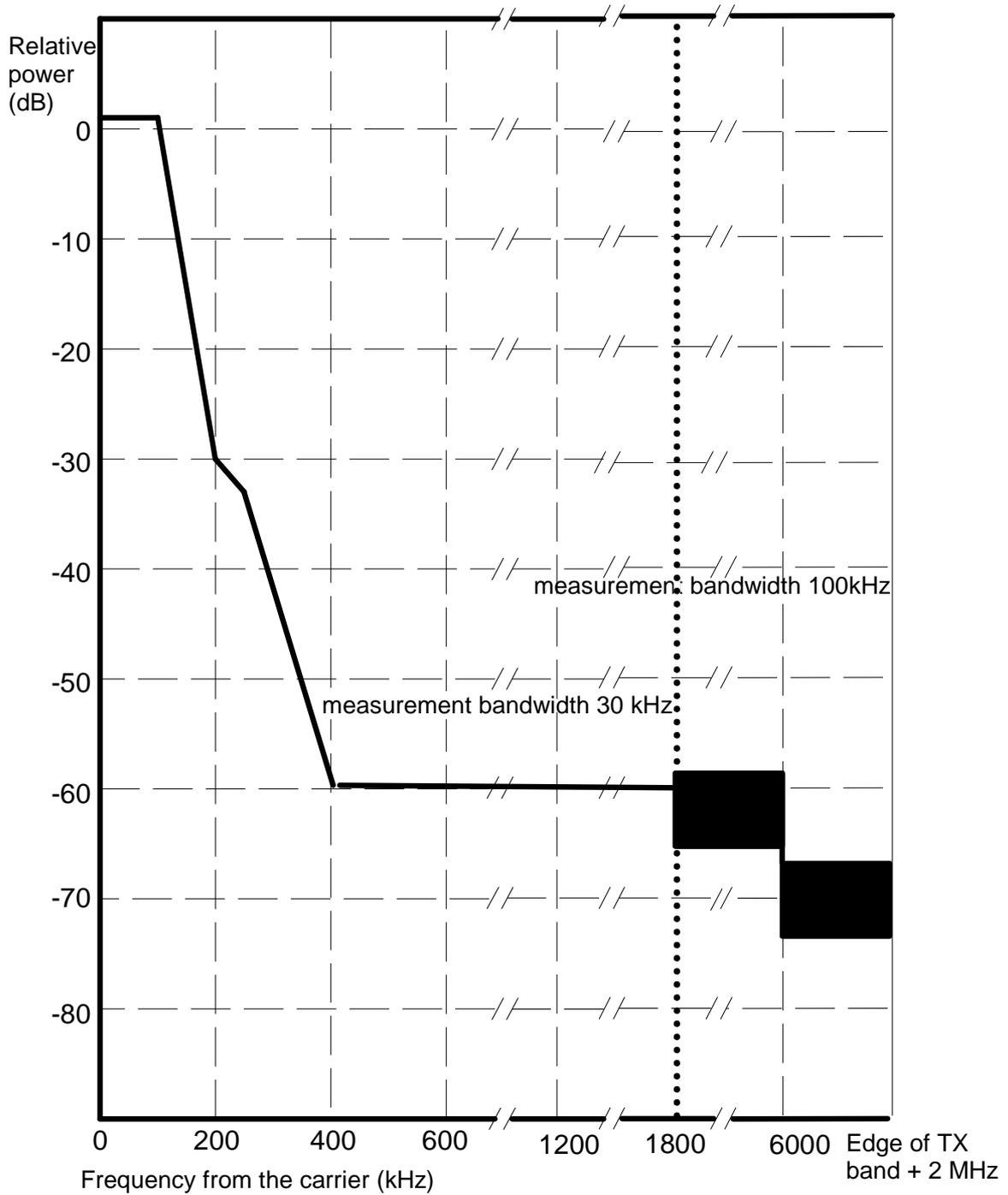
Figure A.2: DCS 1 800 CTS-FP spectrum due to modulation
