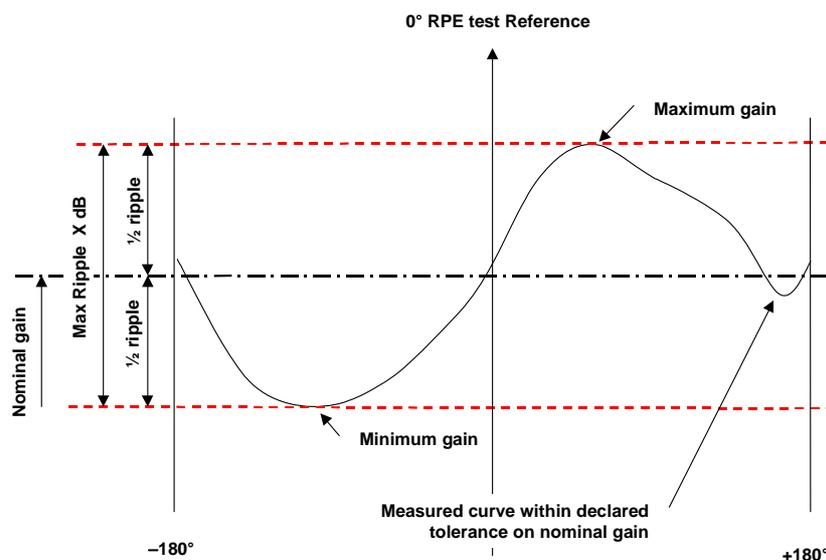
NOTE: Figure 2 shows the relationship between the X dB gain ripple, measured minimum and maximum gains in the azimuth plane, and the declared nominal gain and tolerance of an omnidirectional antenna.
