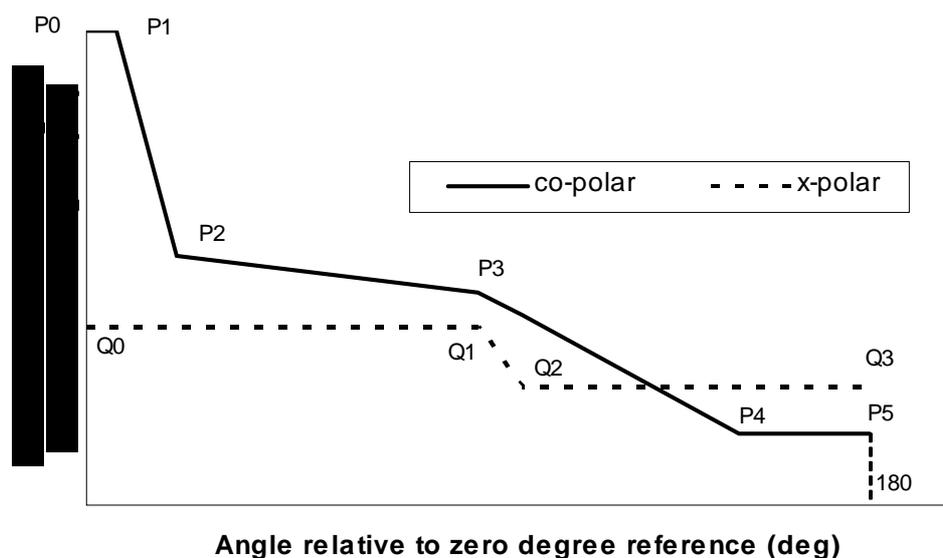
Figure 4: Normalized RPE for DN Azimuth and Elevation
