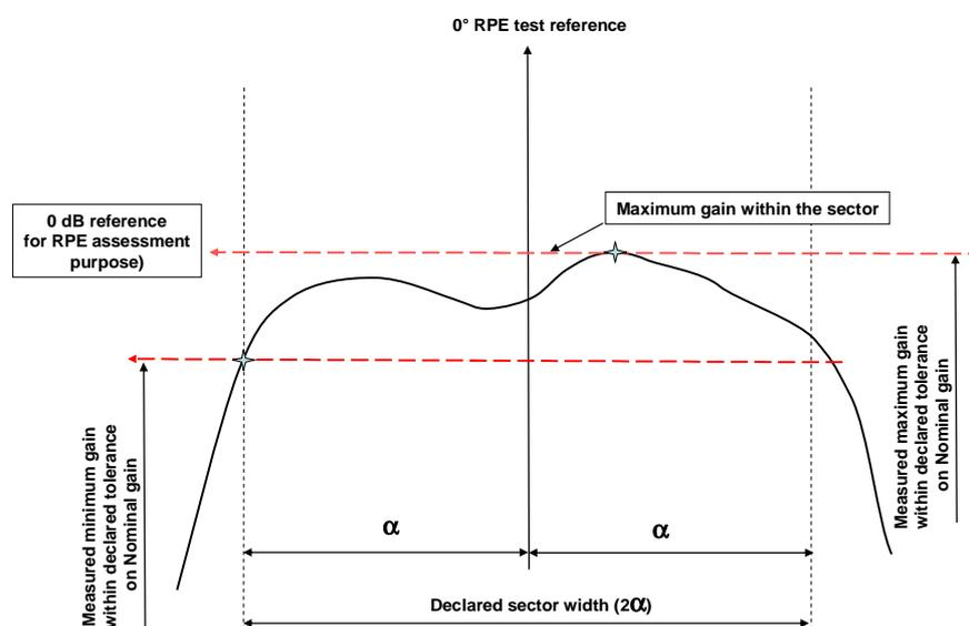
**Figure 3: Gain ripple for a sectored antenna**
