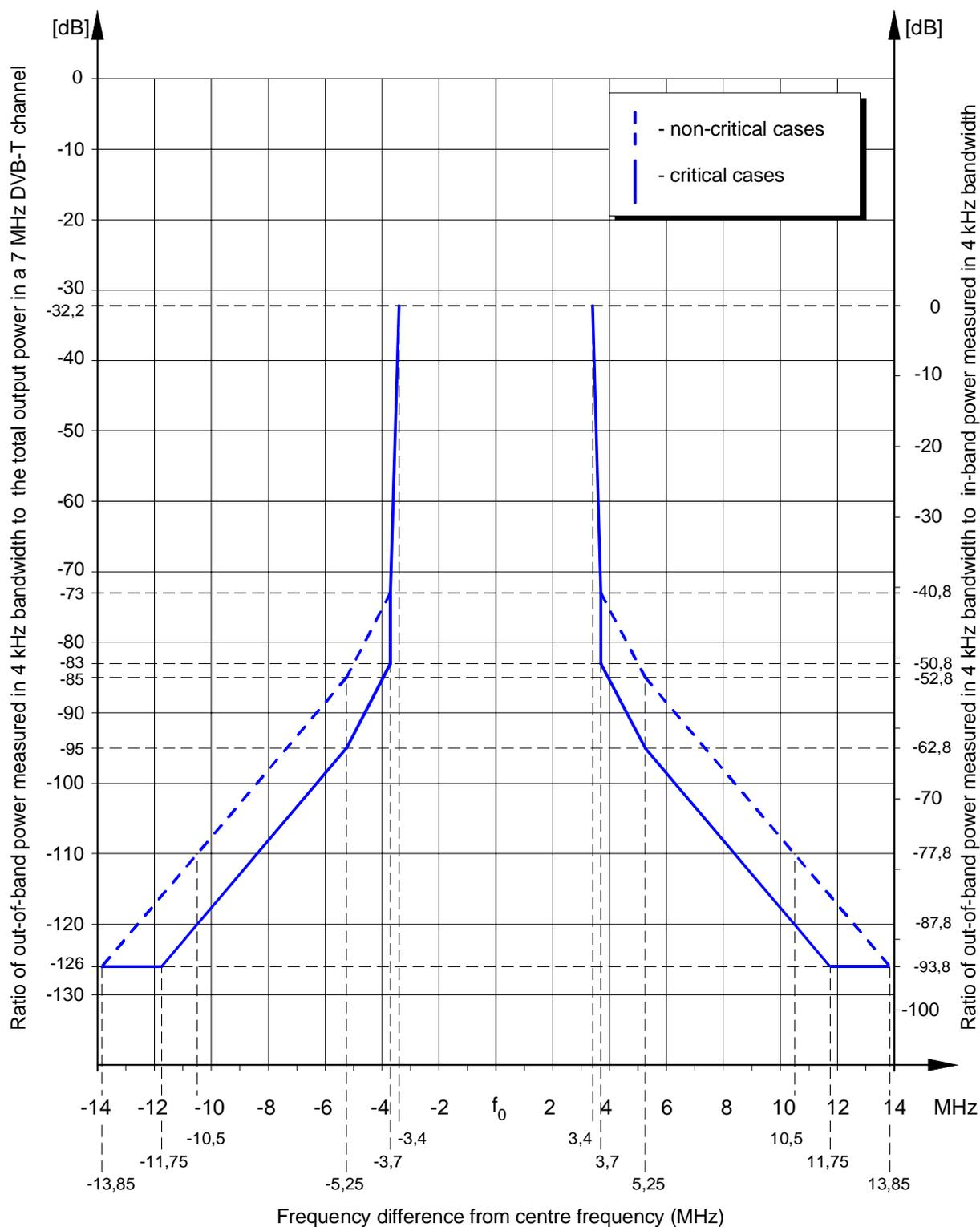
Figure 4.3: Out-of-band limits for DVB-T transmitters  $\geq 25$  W in 7 MHz channels
