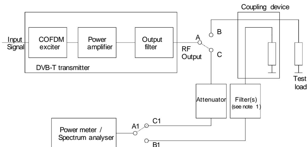
NOTE 1: The optional filter should suppress the output signal so that no intermodulation products are generated by the spectrum analyser. The insertion loss throughout the measuring range should be known.
