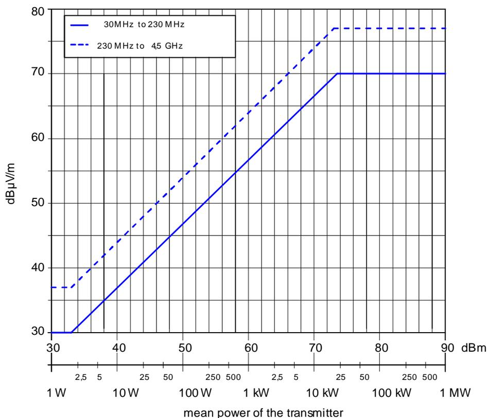
Figure 4.5: Cabinet radiation limits for DVB-T transmitters
