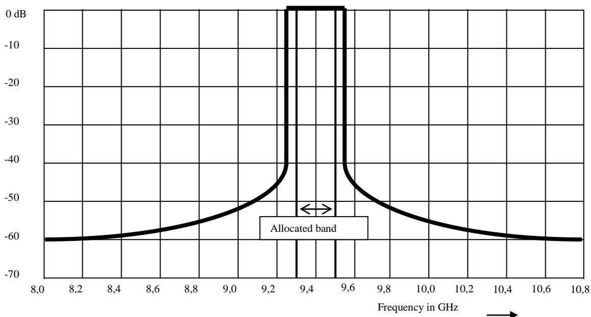
**Figure C.2: Maximum permitted Out Of Band-emissions power level**
