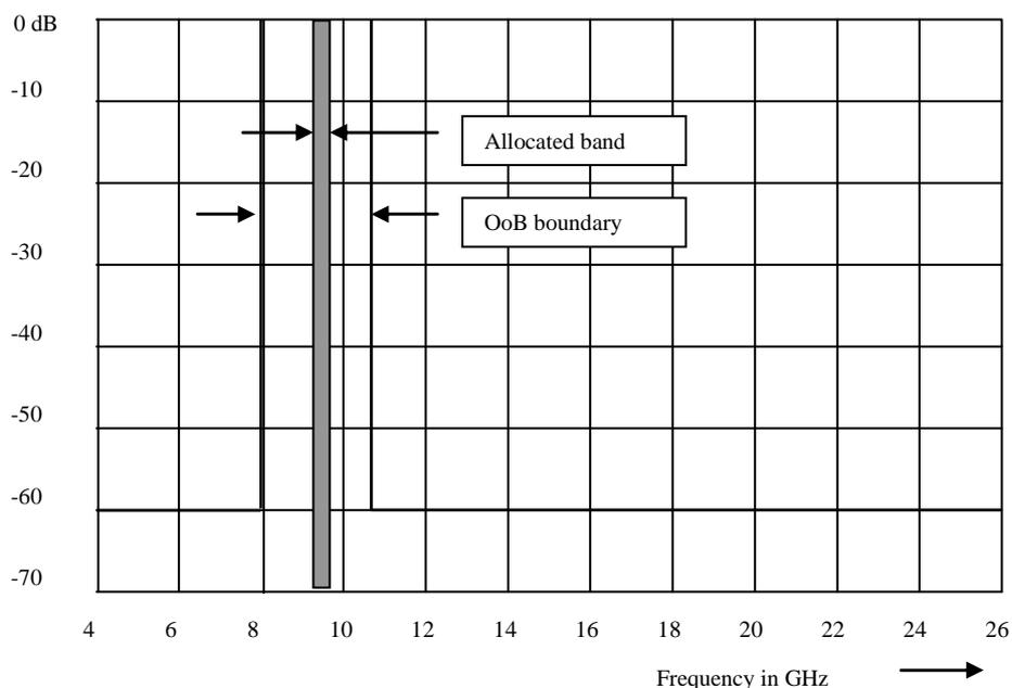
**Figure C.3: Maximum permitted spurious emissions power level**
