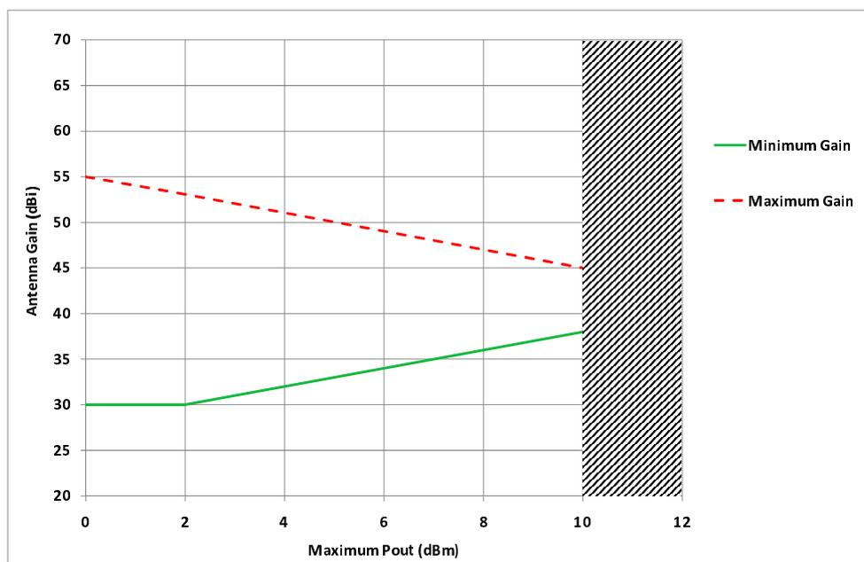
NOTE: For equipment with permanent ATPC feature, the minimum gain is intended evaluated with the maximum Pout delivered by the ATPC regime in unfaded condition, while the maximum gain is intended evaluated with the maximum Pout in full power ATPC regime (see example).
