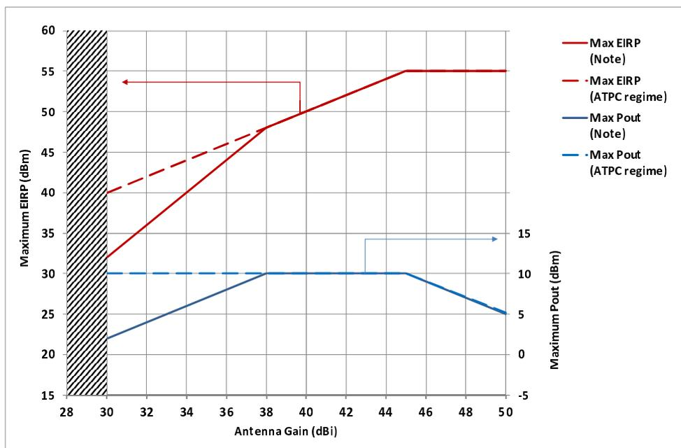
NOTE: For equipment with permanent ATPC feature, these are intended the maximum Pout and EIRP delivered by the ATPC regime in unfaded conditions.
