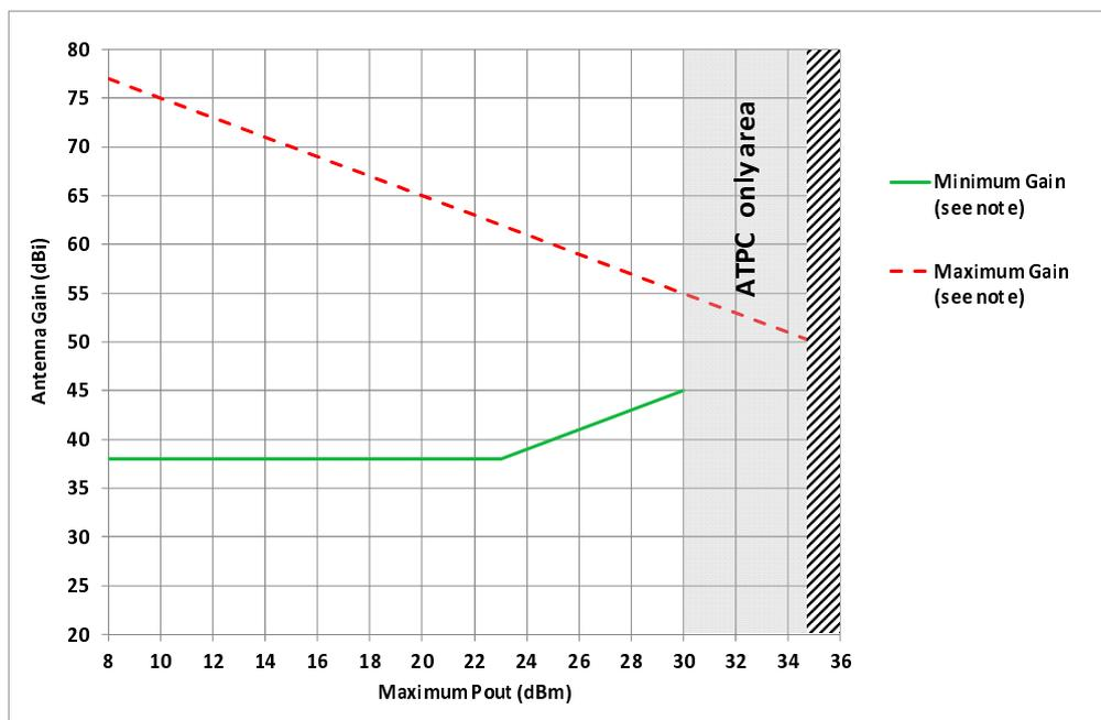
NOTE: For equipment with permanent ATPC feature, the minimum gain is intended evaluated with the maximum Pout delivered by the ATPC regime in unfaded condition, while the maximum gain is intended evaluated with the maximum Pout in full power ATPC regime (see example).
