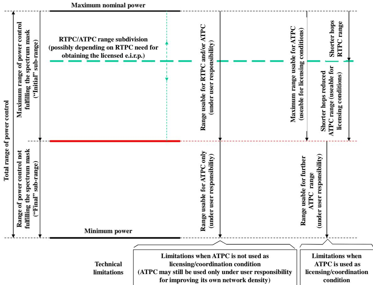
Figure D.3: ATPC/RTPC ranges and licensing/coordination conditions
