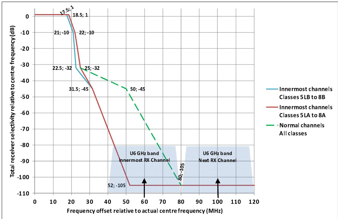
NOTE: The corner points of the main lobe filter are the same of the relevant spectrum masks a part from the +2 dB (K1 value) brought down to 0 dB; see ETSI EN 302 217-2 [18].
