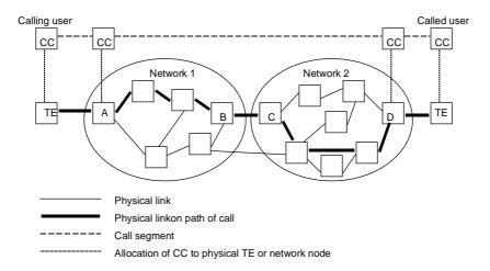
Figure 4: Call originating and terminating in different networks
