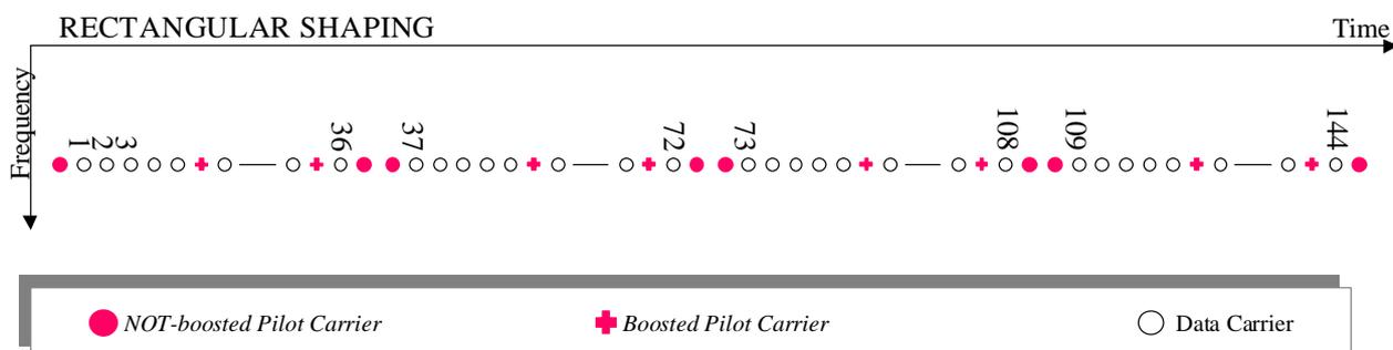
**Figure 23: BS1 with Rectangular shaping and without frequency hopping option**
