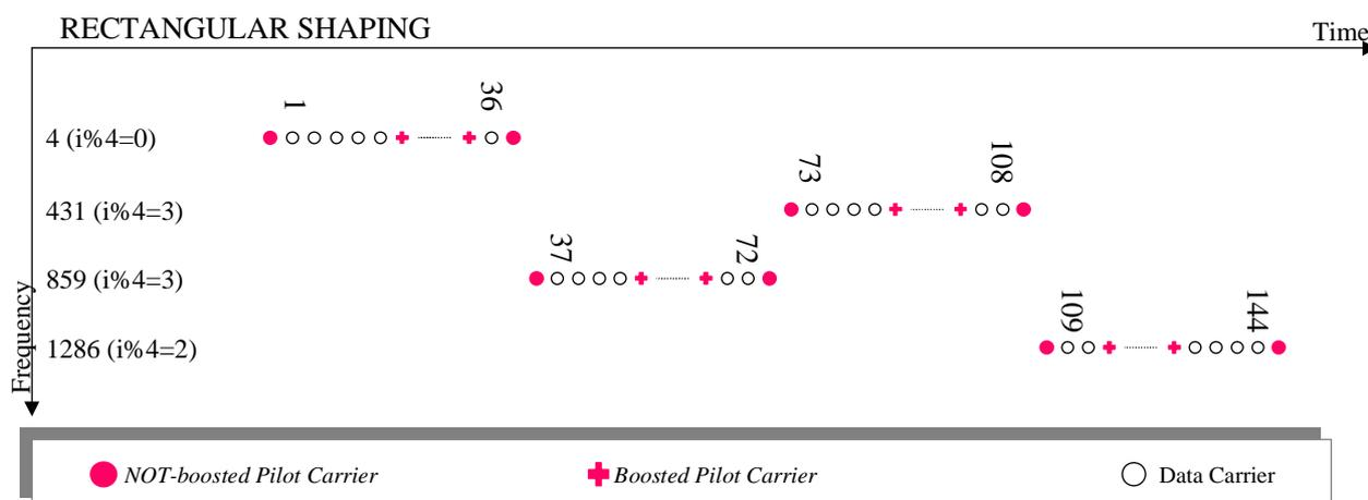
**Figure 25: BS1 with frequency hopping and Rectangular shaping**
