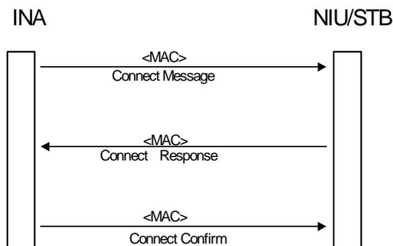
Figure 48: Connection signalling for the initial connection
