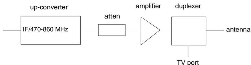
**Figure D.1: RF stage Block Diagram**
