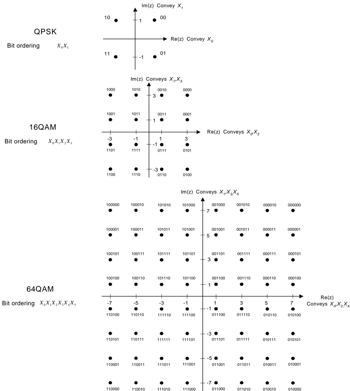
Figure 19: QPSK, 16QAM and 64QAM constellations
