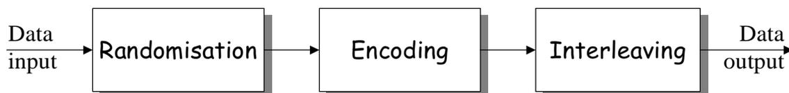
Figure 13: Conceptual diagram of the Return Channel (RC) encoding and interleaving
