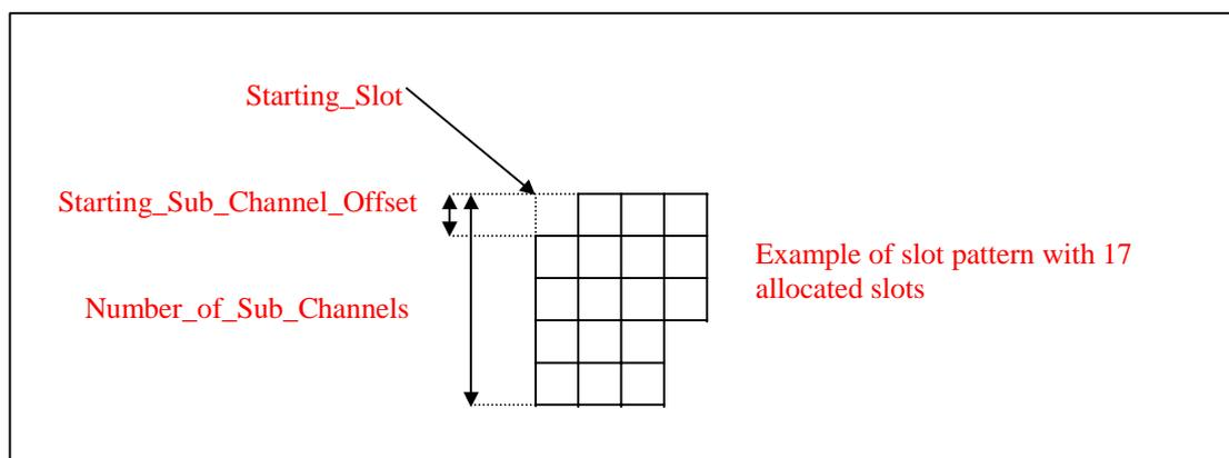
**Figure 49: Slot Pattern structure**
