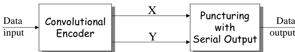
Figure 16: Convolutional encoder block diagram
