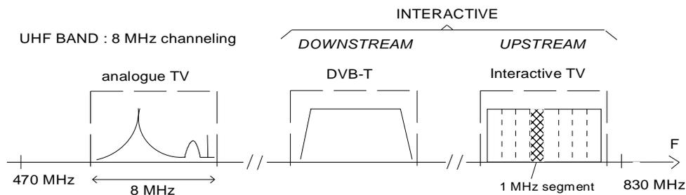
Figure A.1: Sharing of Return Channel spectrum within UHF Broadcasting Bands
