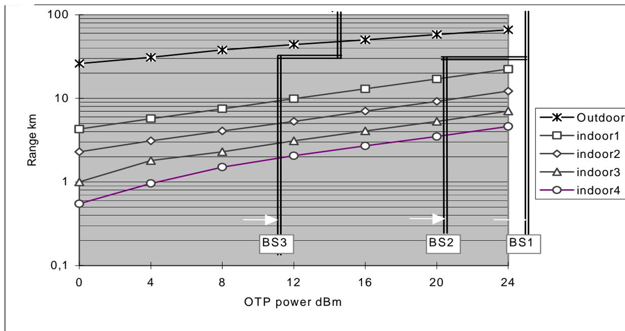
**Figure B.1: Service ranges/transmission power for BS1, BS2 and BS3**
