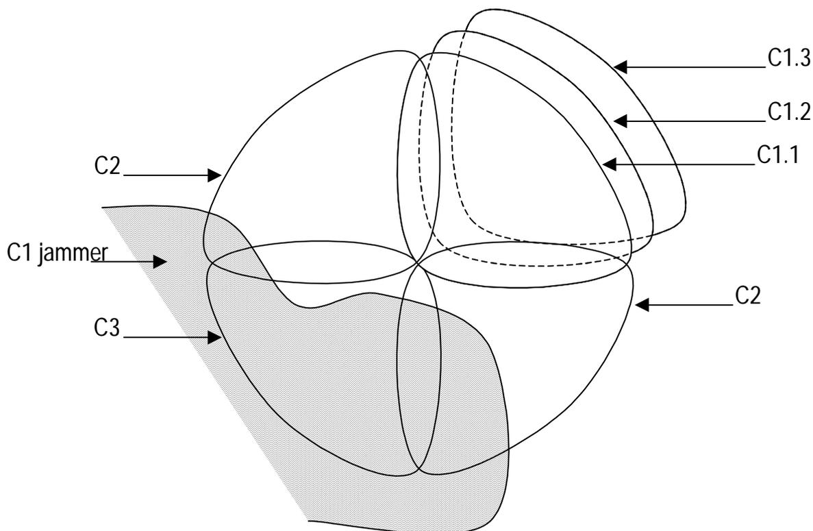
**Figure 43: Sectoring a DVB-T cell; frequency re-use; minimizing interference; several US channels inside one sector**
