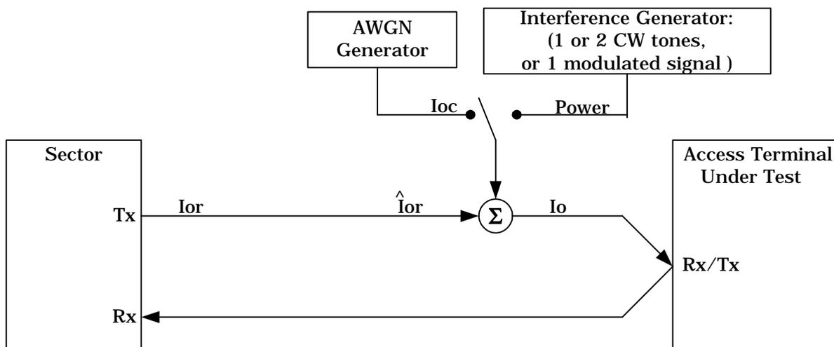
Figure D.5.1-4: Functional Set-up for Tests without Fading
