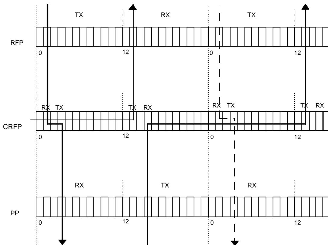
Figure 4: Typical frame multiplexing structure of the CRFP
