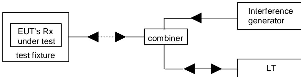
**Figure 13: Measuring arrangement for calibration**
