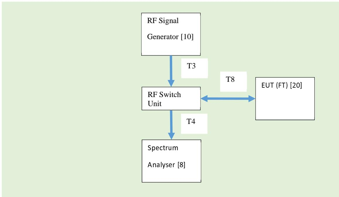
**Figure 37: FT Test Setup**
