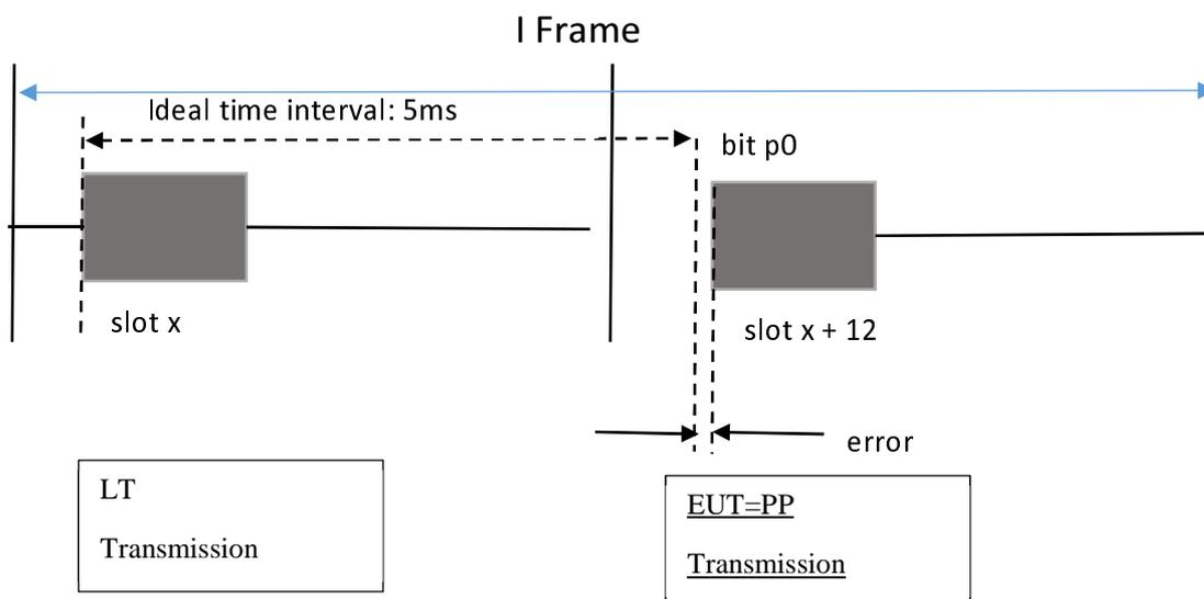
Figure 30: PP packet transmission error definition
