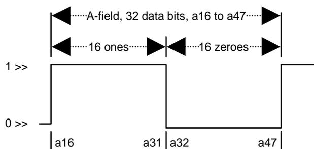
Figure 32: Test packet structure for case 2, A-field
