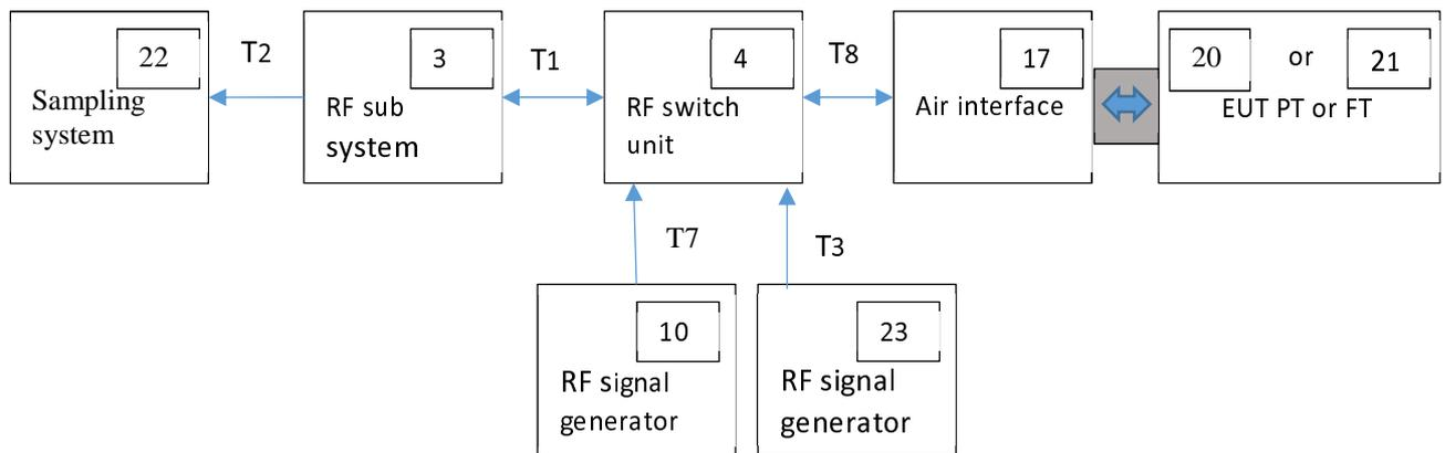
Figure 17: Test setup 3
