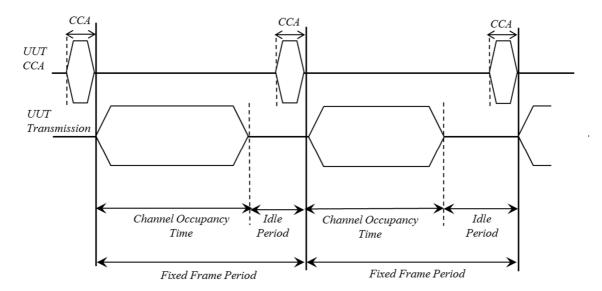
Figure 2: Example of timing for Frame Based Equipment
