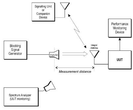
Figure C.4: Measurement Set-up
