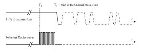
Figure 12: Example of timing for radar testing during In-Service Monitoring
