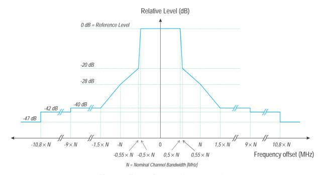
Figure 1: Transmit spectral power mask
