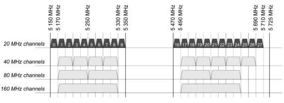
Figure 3: Channel Bonding for option 2
