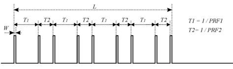
Figure D.3: General structure of a single burst/single pulse based staggered PRF radar test signal
