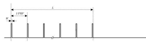
Figure D.1: General structure of a single burst/constant PRF based radar test signal
