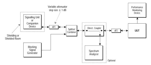
Figure 18: Test Set-up for receiver blocking
