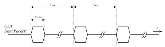
Figure 4: General structure of the test transmission sequences
