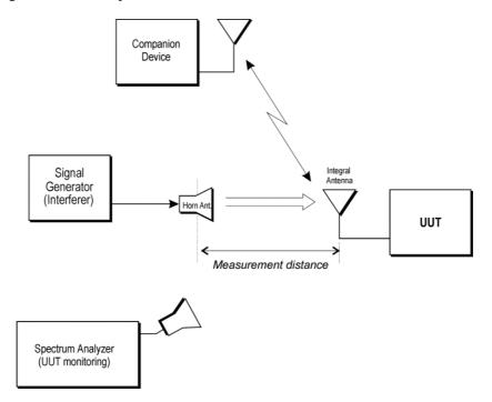
Figure C.2: Measurement Set-up
