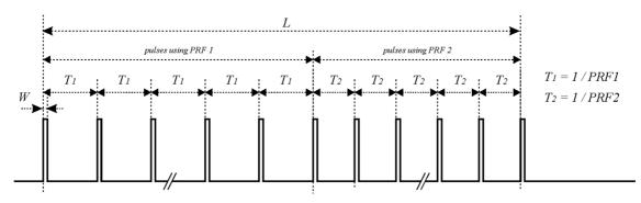
Figure D.4: General structure of a single burst/packet based staggered PRF radar test signal
