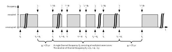
Figure 17: Example of UUT transmissions
