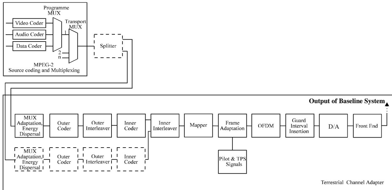
Figure 1: Functional block diagram of the Baseline System
