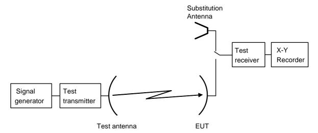
Figure 8: Test arrangement-antenna transmit gain measurement
