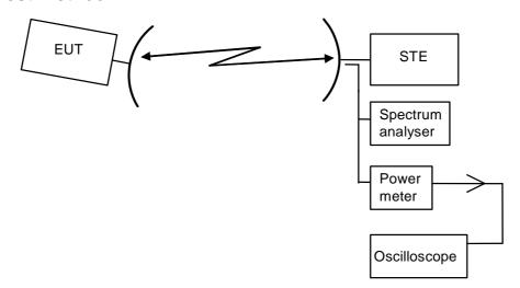
Figure 10: Test arrangement for pointing error detection
