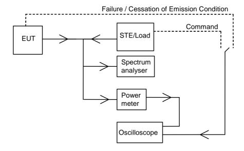
Figure 12: General test arrangement for control and monitoring tests for conducted measurements
