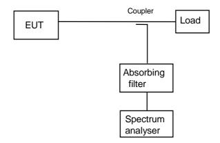
Figure 5: Test arrangement - on-axis spurious radiation measurements at the antenna flange
