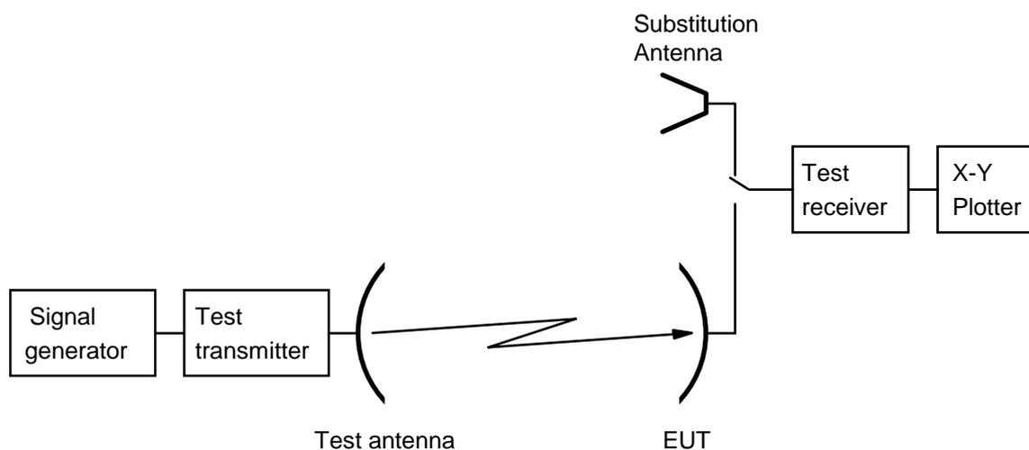
**Figure 10: Test arrangement - antenna transmit gain measurement**
