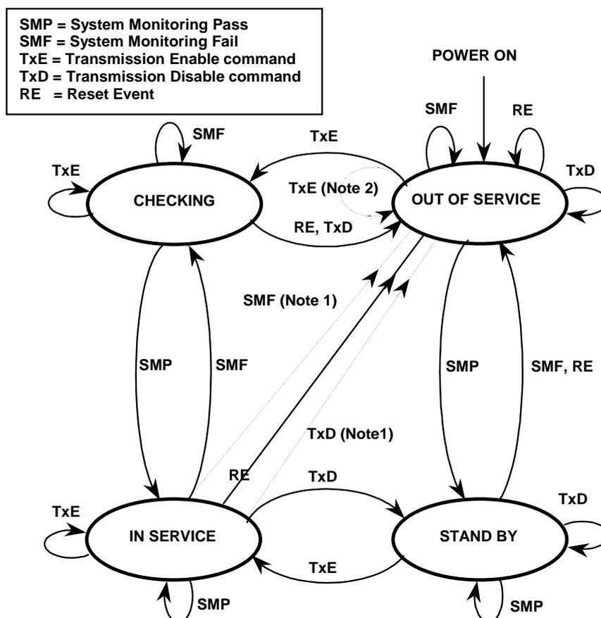
NOTE 1: In the "in-service" state, the occurrence of a SMF and/or TxD may result in a transition to the "out-of-service" state.
