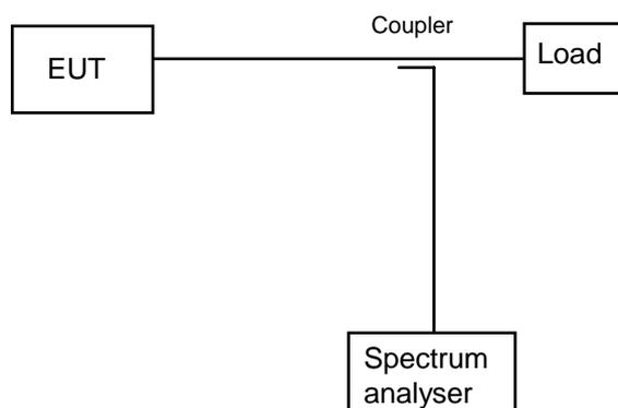
**Figure 9: Test arrangement - transmit output power density measurement**
