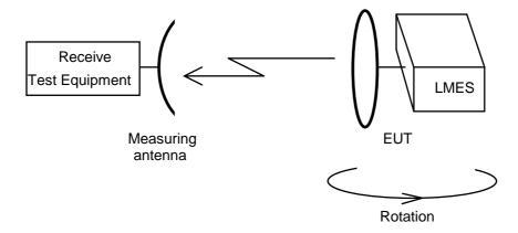
Figure 2: Test arrangement - Unwanted emissions measurement, first axis
