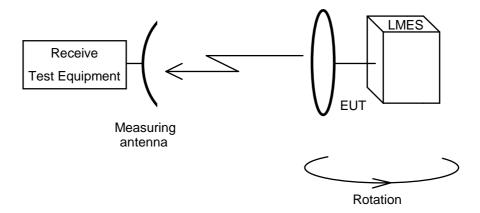
Figure 3: Test arrangement - Unwanted emissions measurement, second axis
