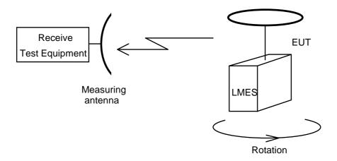
Figure 4: Test arrangement - Unwanted emissions measurement, third axis
