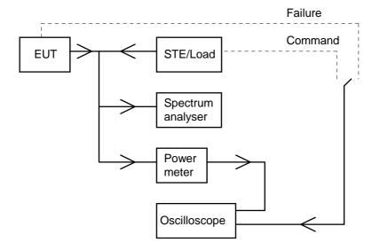
Figure 6: General test arrangement for control and monitoring tests for conducted measurements
