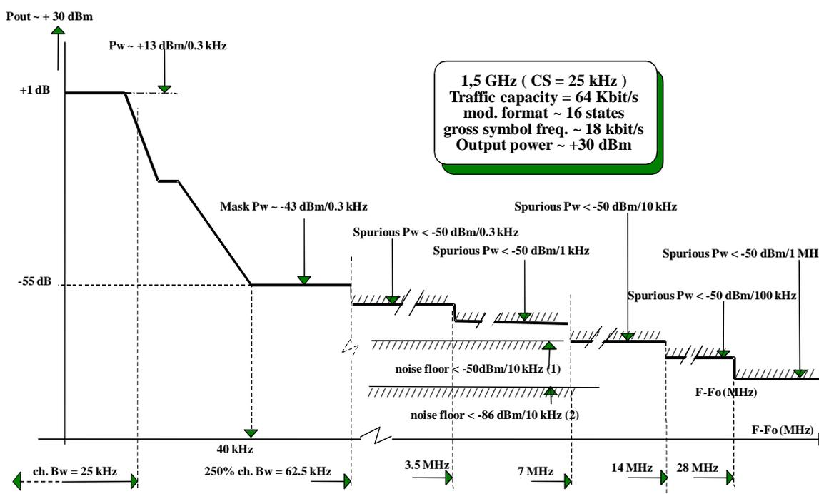
NOTE 1: Typical noise floor with 3<sup>rd</sup> order i.m.p.  $> 50\text{ dB}$ .
