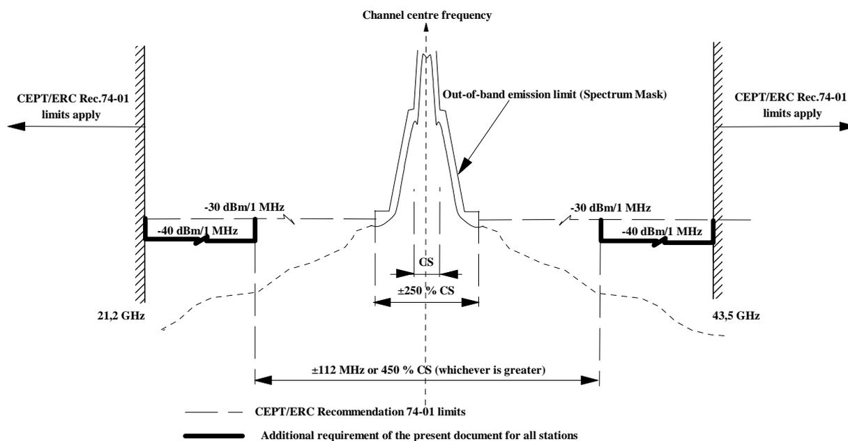
Figure 3: MP equipment for channel separation  $CS > 10$  MHz
