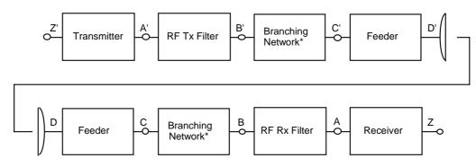
NOTE 1: For the purpose of defining the measurement points, the branching network does not include a hybrid. NOTE 2: Points B and C, B' and C' may coincide.
