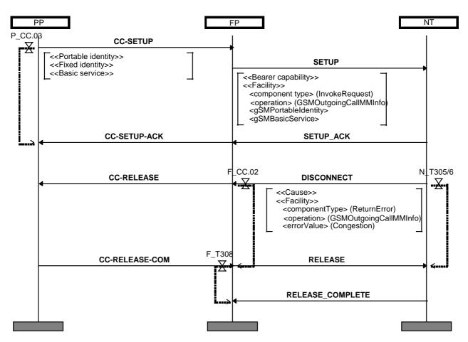
Figure 12: Outgoing call failure, e.g. no resources in network
