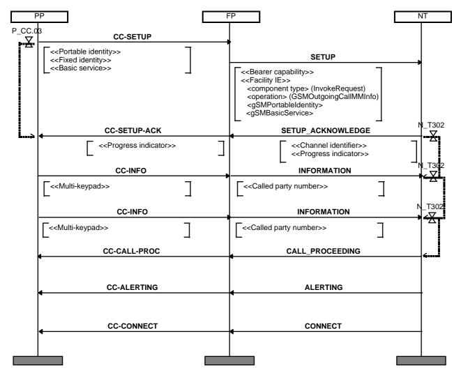
NOTE: Authentication and ciphering may be done in parallel to call establishment. The network may delay sending of SETUP\_ACK until completion of ciphering.
