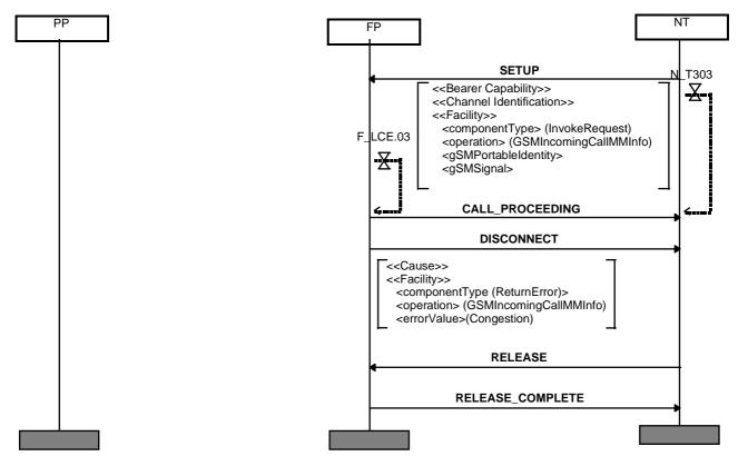
Figure 14: Incoming call failure, FT resources unavailable
