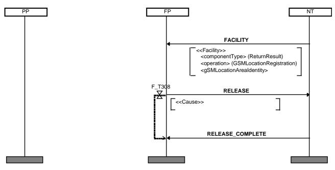
NOTE: Terminal initiated MM-signalling connection release. Only used in exceptional cases e.g. maintenance action.
