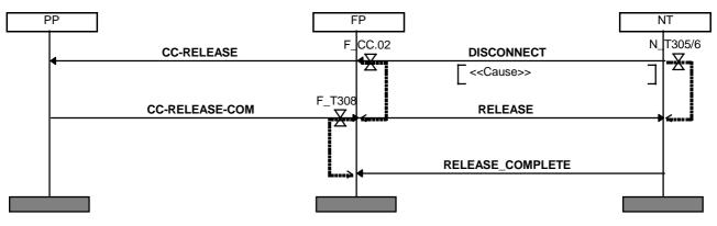
Figure 16: Normal call release, network initiated
