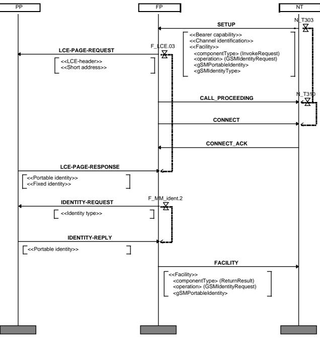
NOTE: This is the normal network initiated NCICs connection establishment. IdentityRequest operation is given as an example.
