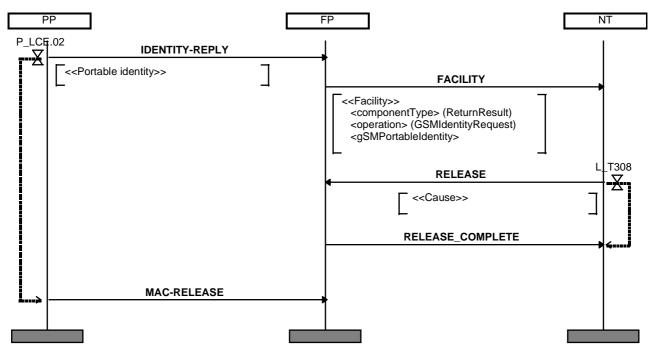
NOTE: Identity request is given as an example. Partial release applies at the air interface.
