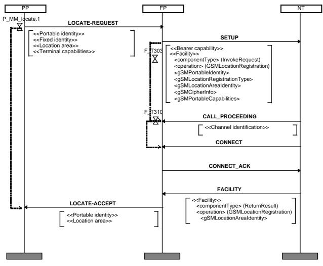
NOTE: This is the normal terminal initiated NCICs connection establishment. The Location Registration operation is given as an example.
