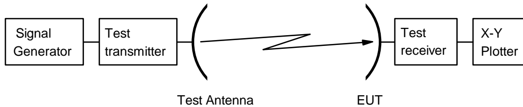
Figure 10: Test arrangement - antenna transmit radiation pattern measurement
