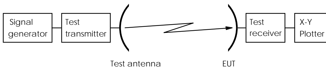
Figure 10: Test arrangement - transmit polarization discrimination
