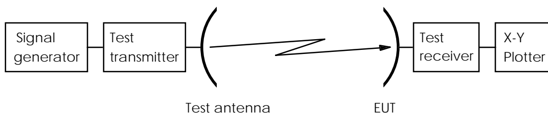
Figure 10: Test arrangement - transmit polarization discrimination
