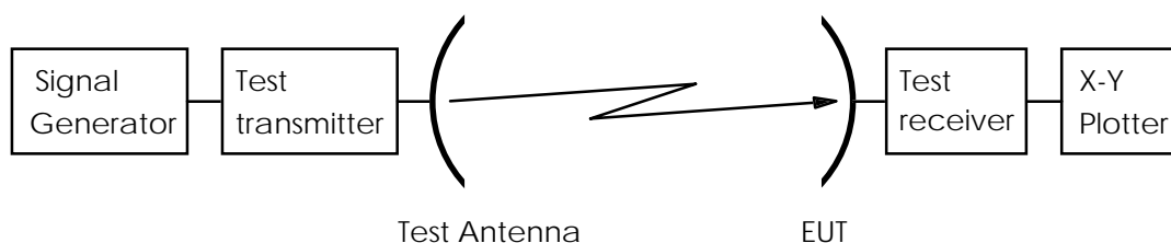
Figure 9: Test arrangement - antenna transmit radiation pattern measurement
