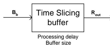
Figure 18: The Time Slicing/MPE-FEC buffer in the Receiver
