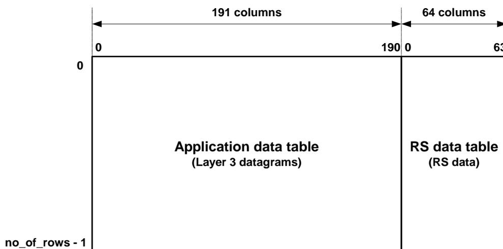
Figure 13: The structure of the MPE-FEC Frame
