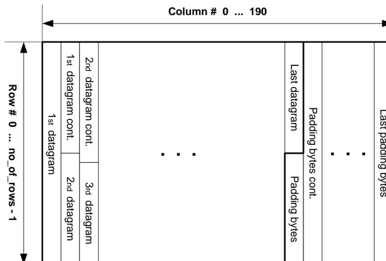
Figure 15: The layout of the Application data table
