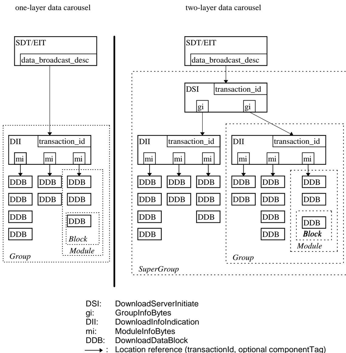
**Figure 21: Structure of the DVB data carousel**
