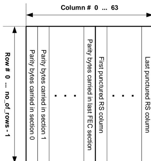
Figure 16: The layout of the RS data table
